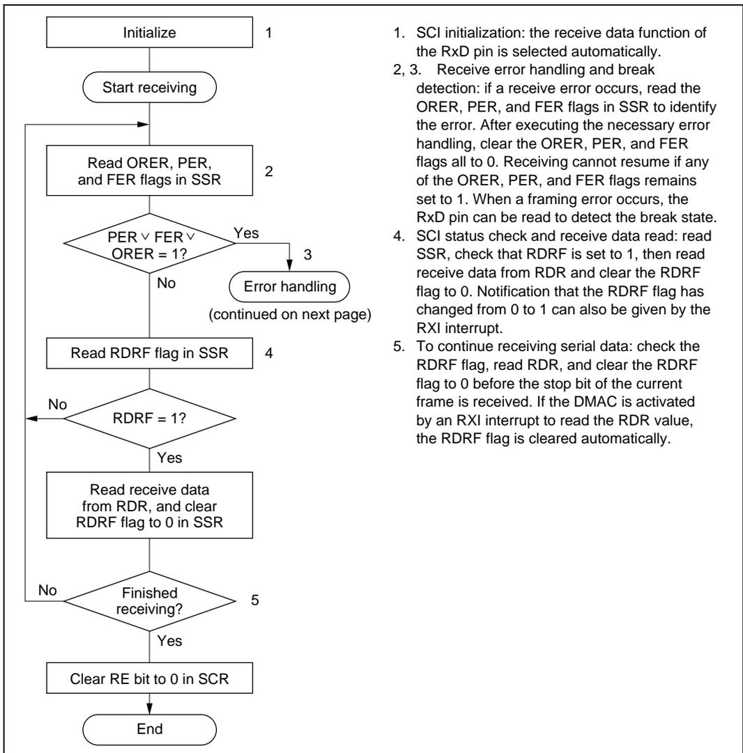
1. SCI initialization: the receive data function of the RxD pin is selected automatically.
