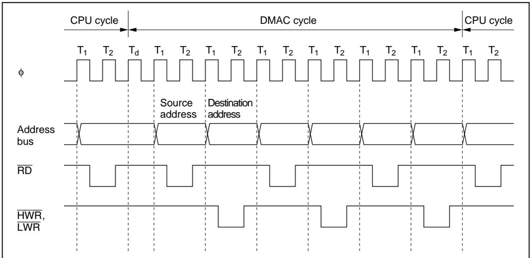
**Figure 8.15 Bus Timing of Burst Mode DMA Transfer**
