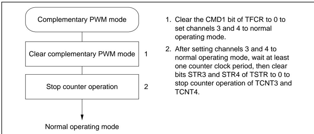
**Figure 10.34** Clearing Procedure for Complementary PWM Mode
