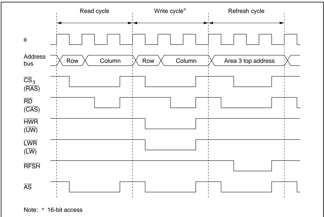
**Figure 7.5(1) DRAM Control Signal Output Timing ( $2\overline{\text{WE}}$  Mode)**
