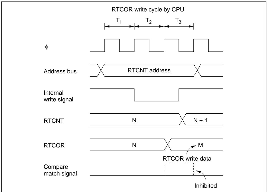
**Figure 7.22** Contention between RTCOR Write and Compare Match
