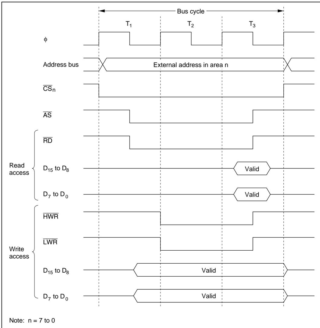
**Figure 6.8 Bus Control Signal Timing for 16-Bit, Three-State-Access Area (3)
