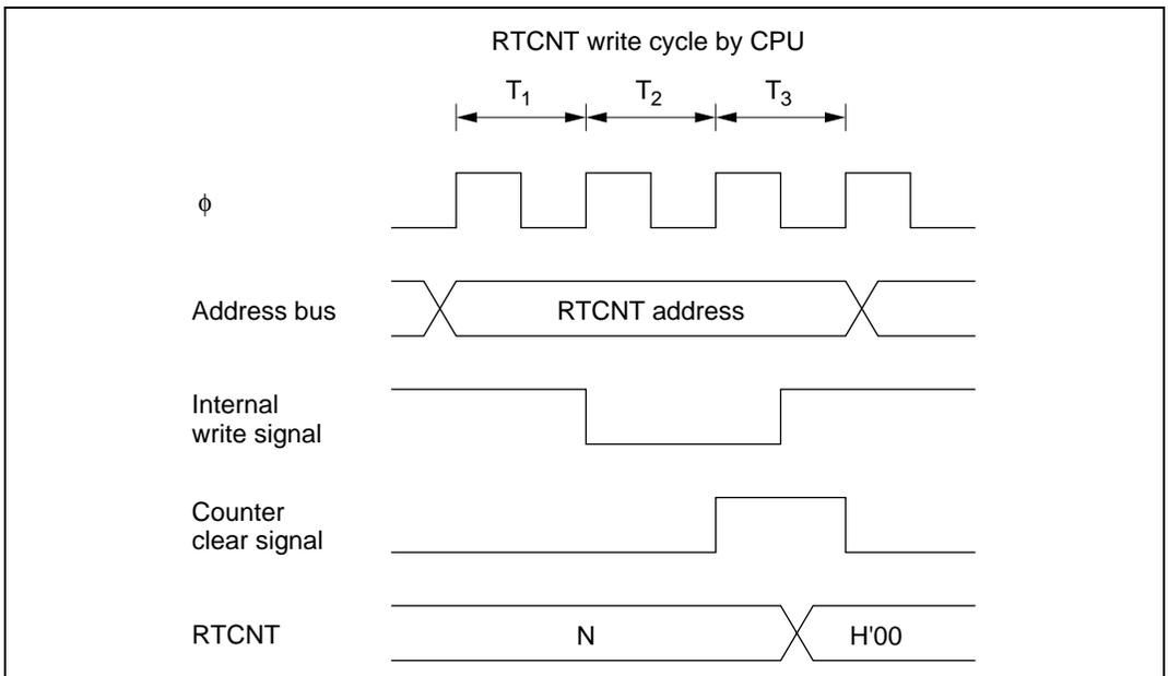
**Figure 7.20** Contention between RTCNT Write and Clear
