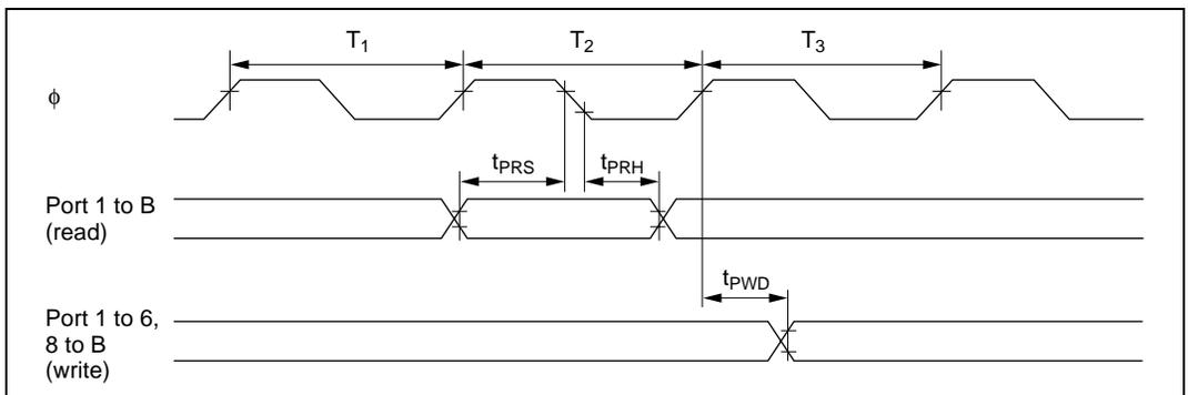
Figure 21.23 TPC and I/O Port Input/Output Timing
