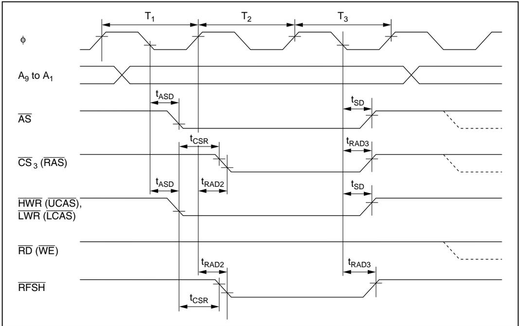
**Figure 21.14 DRAM Bus Timing (Refresh Cycle): Three-State Access**
