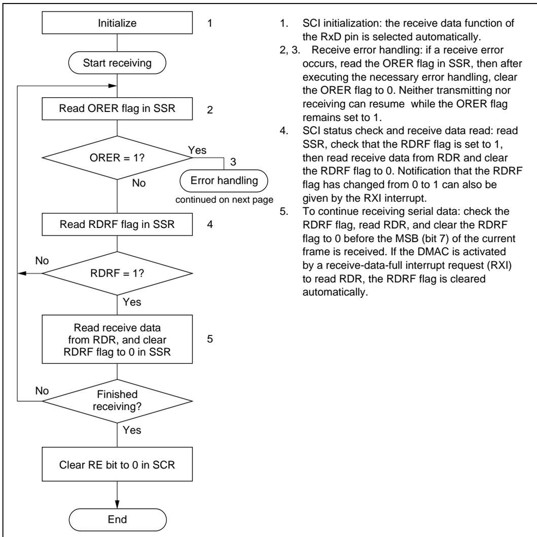
**Figure 13.18 Sample Flowchart for Serial Receiving (1)**
