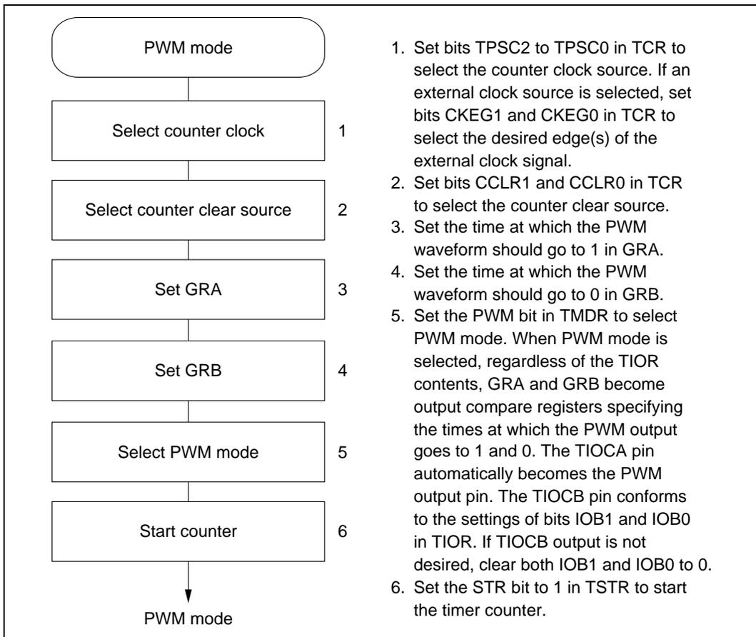
**Figure 10.28 Setup Procedure for PWM Mode (Example)**
