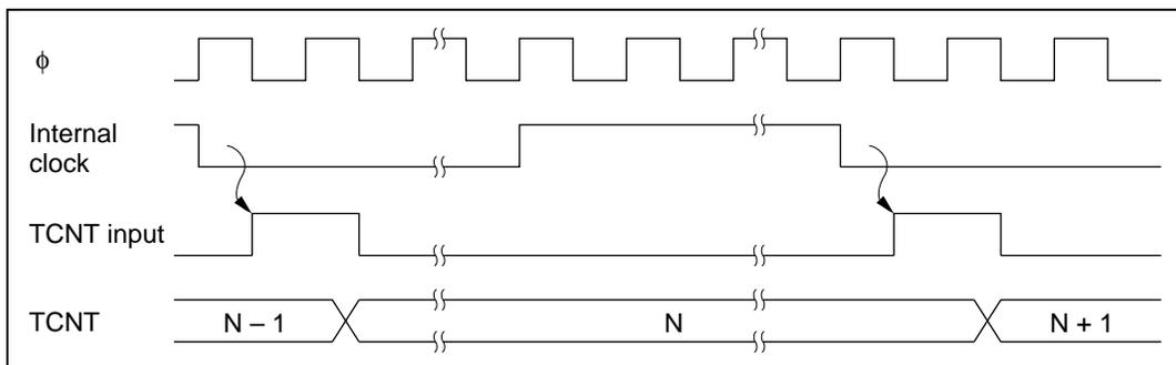
**Figure 10.17 Count Timing for Internal Clock Sources**
