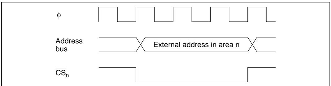
**Figure 6.3  $\overline{CS}_n$  Output Timing ( $n = 7$  to  $0$ )**
