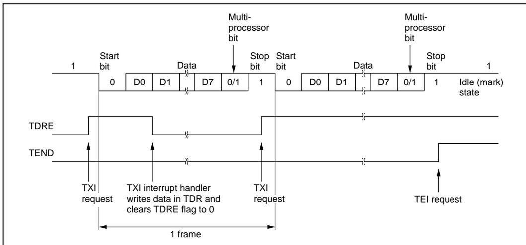
**Figure 13.11 Example of SCI Transmit Operation
