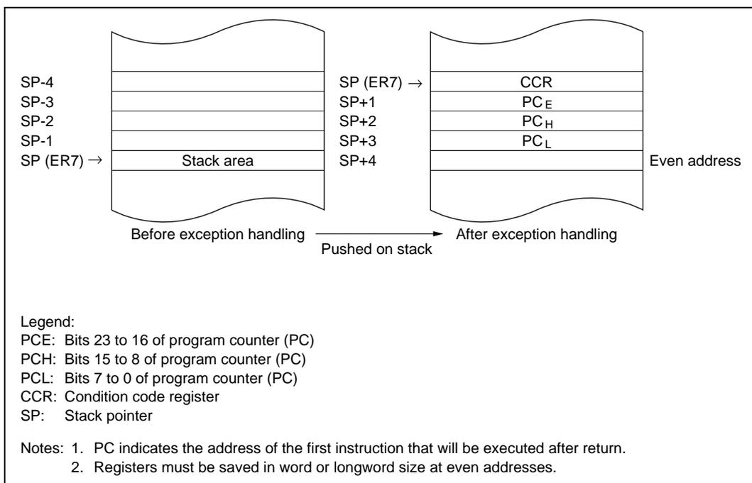
**Figure 4.6 Stack after Completion of Exception Handling**
