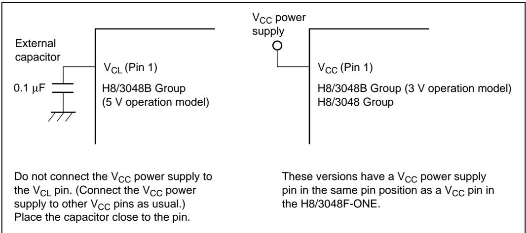
**Figure 1.4 Method of Connecting H8/3048B Group  $V_{CL}$  Capacitor**
