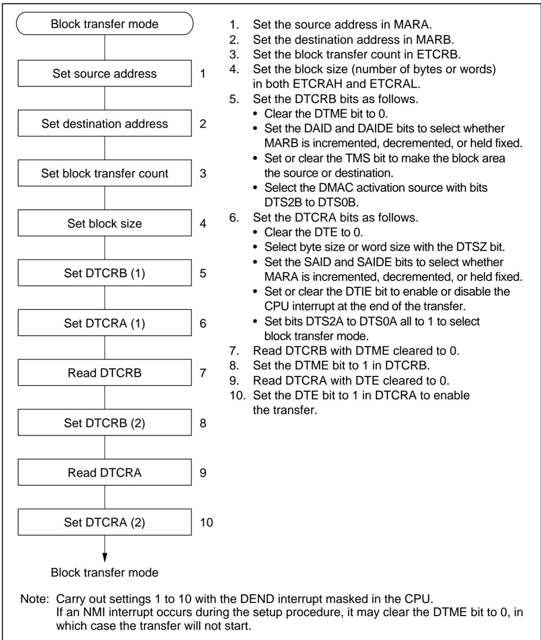
**Figure 8.12 Block Transfer Mode Setup Procedure (Example)**
