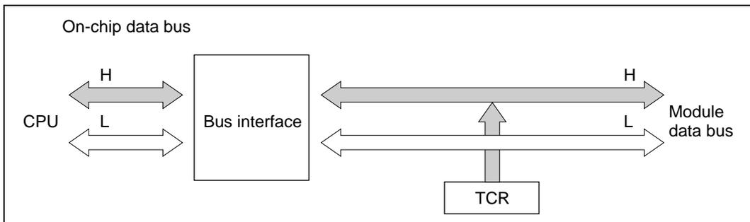
**Figure 10.13 Access to Timer Counter (CPU Reads TCR)**
