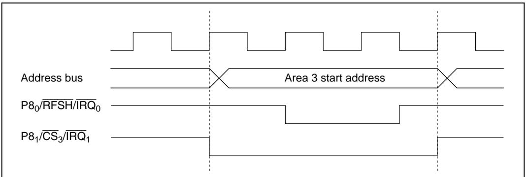
**Figure 7.23 Operation when DRAM/PSRAM Connection Is Switched**
