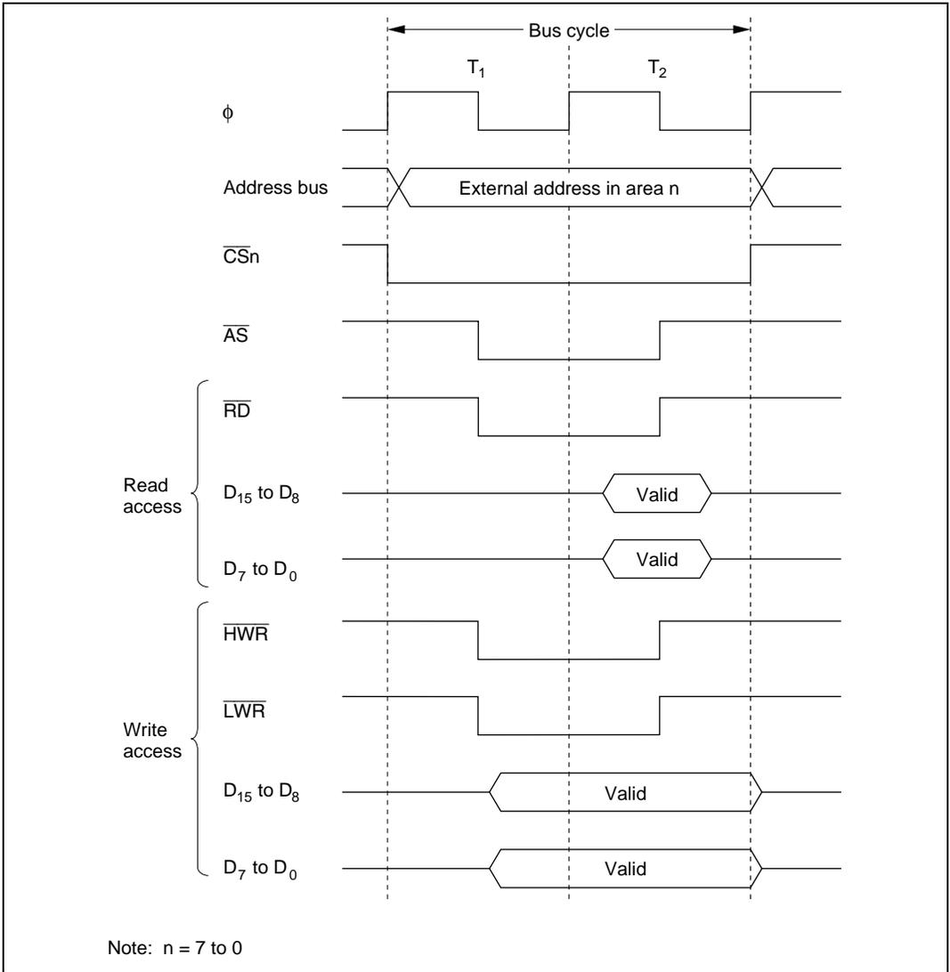
**Figure 6.11 Bus Control Signal Timing for 16-Bit, Two-State-Access Area (3)
