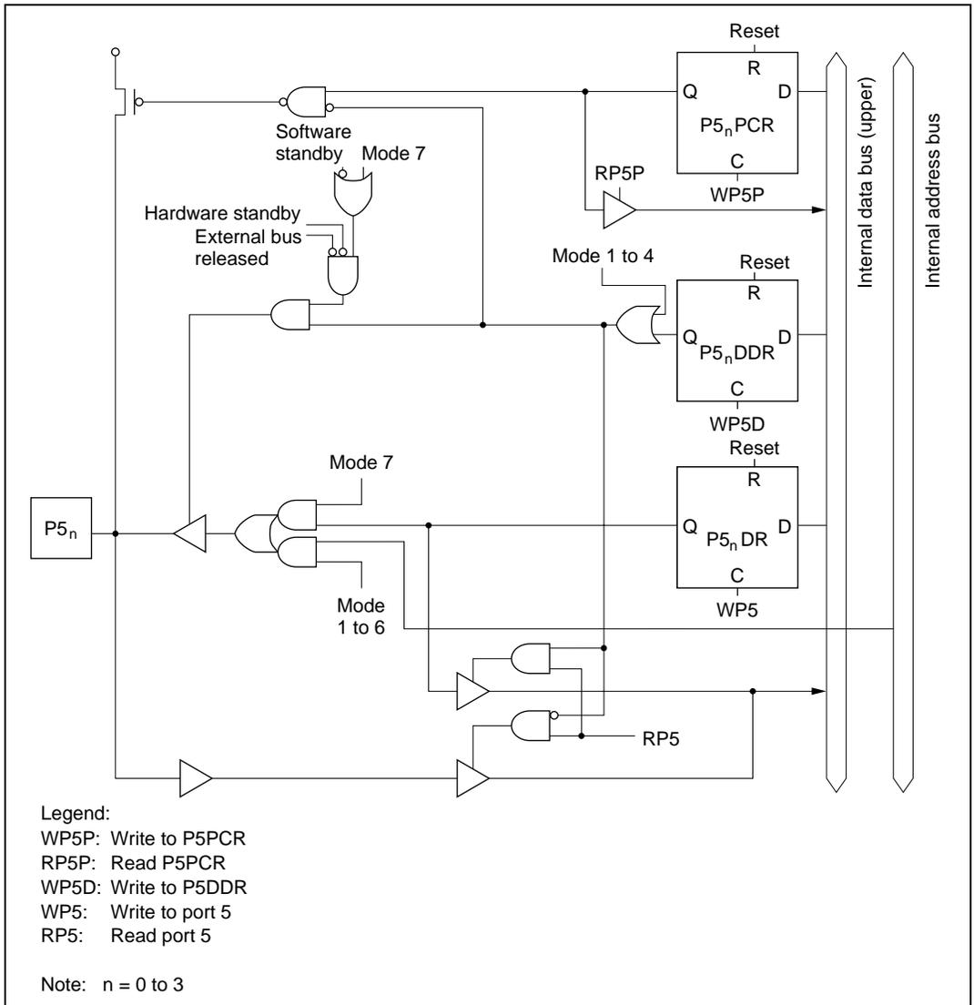
**Figure C.5 Port 5 Block Diagram (Pins P5<sub>0</sub> to P5<sub>3</sub>)**
