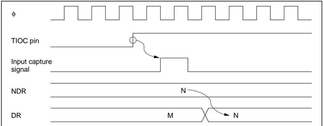
Figure 11.8 TPC Output Triggering by Input Capture (Example)
