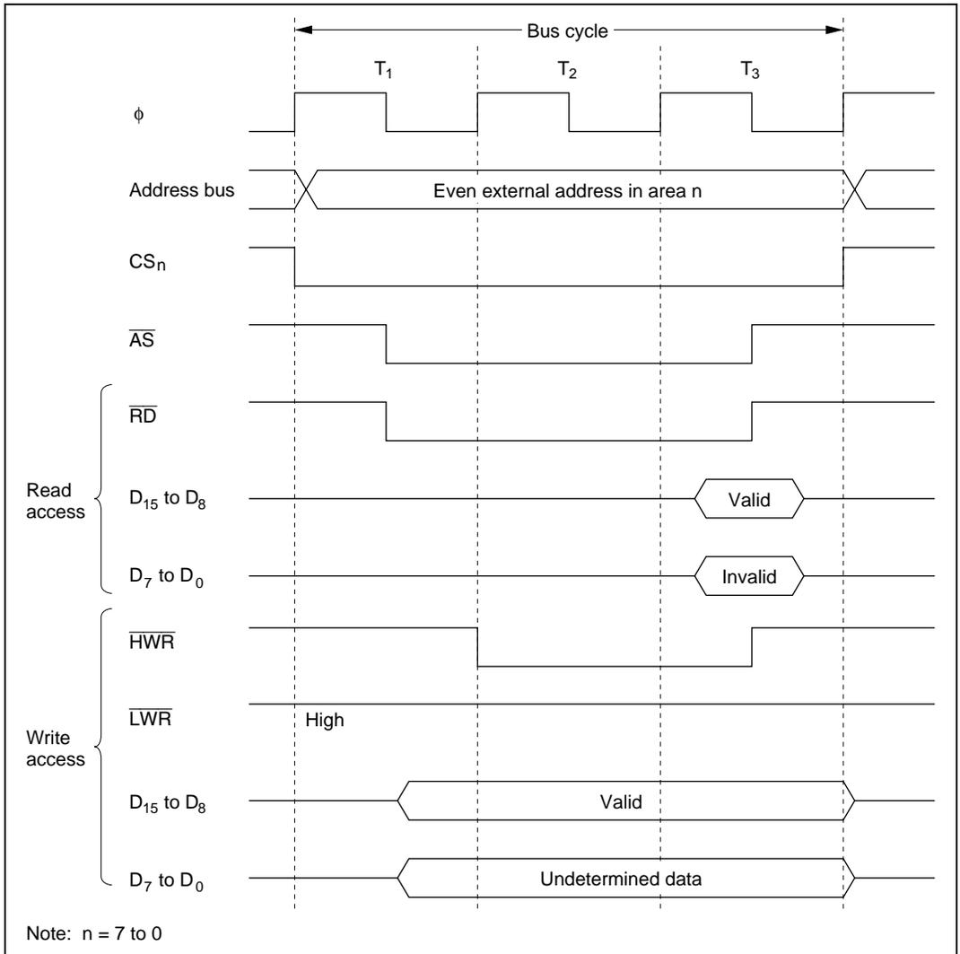
**Figure 6.6 Bus Control Signal Timing for 16-Bit, Three-State-Access Area (1)**
