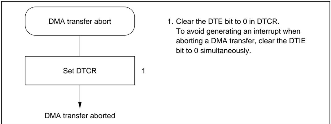
**Figure 8.22 Procedure for Aborting a DMA Transfer**
