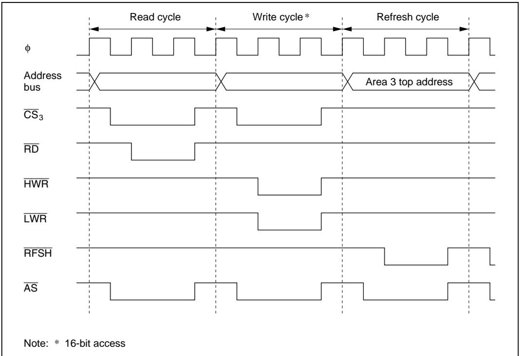
**Figure 7.15 Pseudo-Static RAM Control Signal Output Timing**
