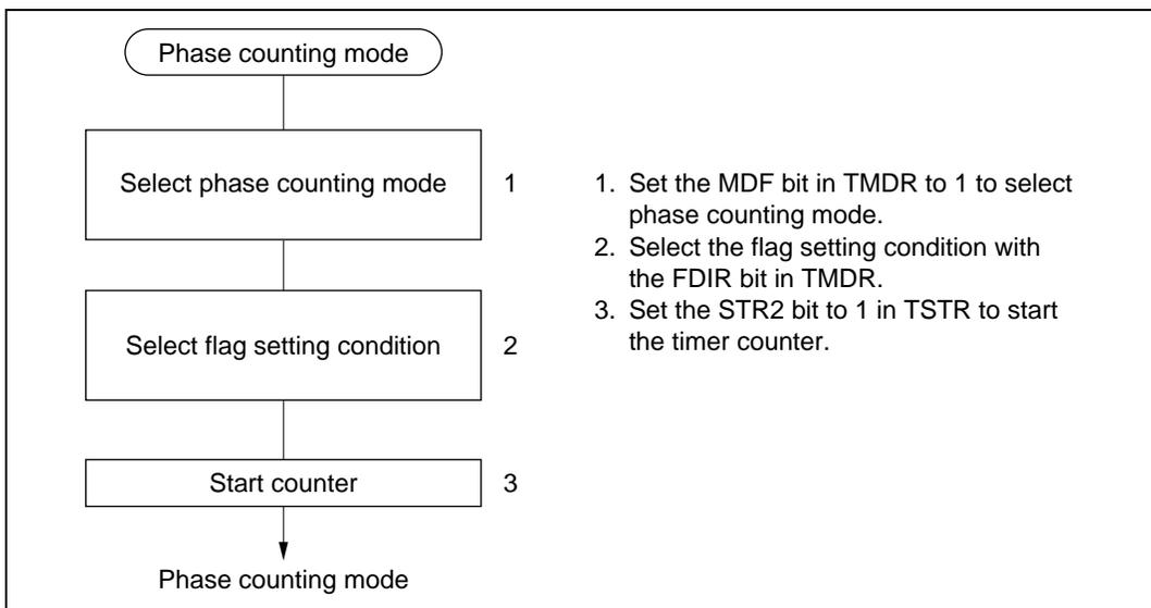
**Figure 10.43 Setup Procedure for Phase Counting Mode (Example)**
