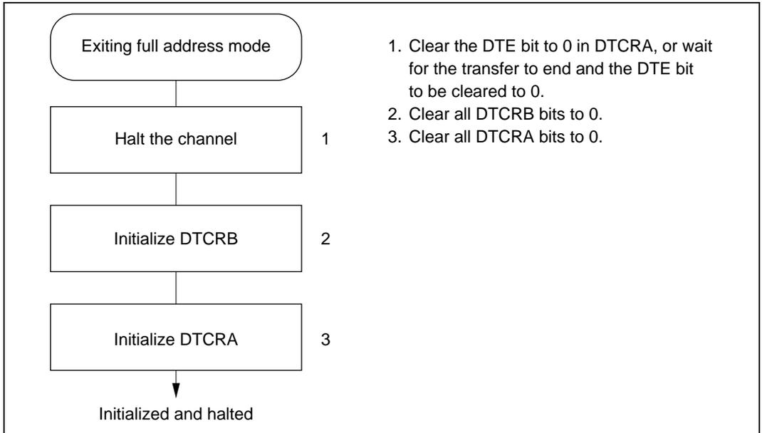
**Figure 8.23 Procedure for Exiting Full Address Mode (Example)**
