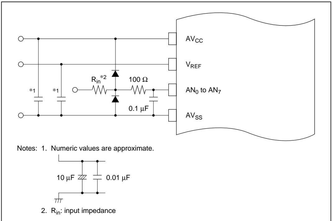
**Figure 15.7 Example of Analog Input Protection Circuit**
