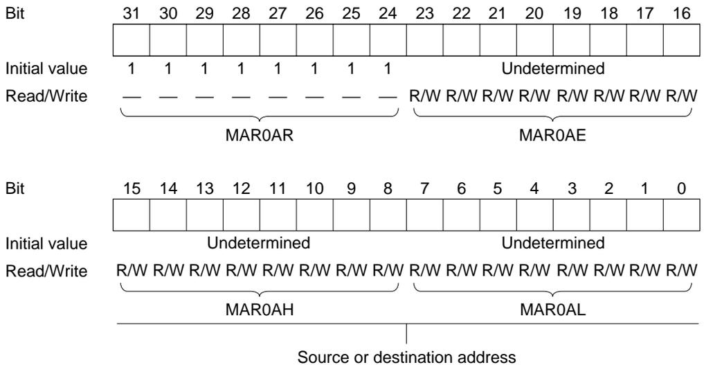
**ETCR0A H/L—Execute Transfer Count Register 0A H/L****H'24, H'25****DMAC0**
