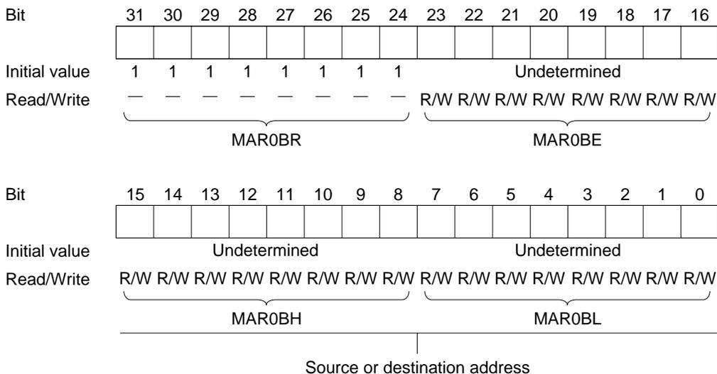
**ETCR0B H/L—Execute Transfer Count Register 0B H/L****H'2C, H'2D****DMAC0**
