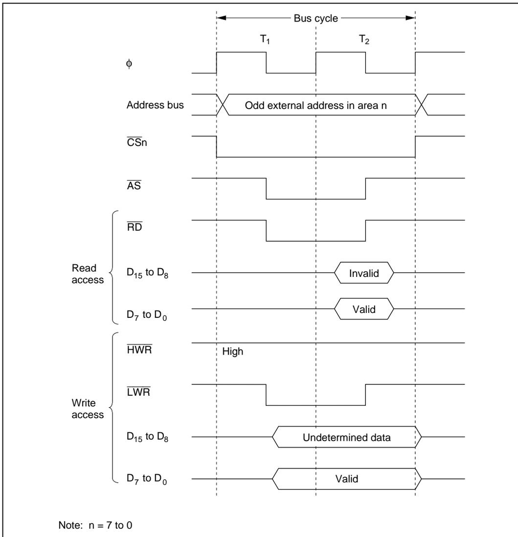
**Figure 6.10 Bus Control Signal Timing for 16-Bit, Two-State-Access Area (2)
