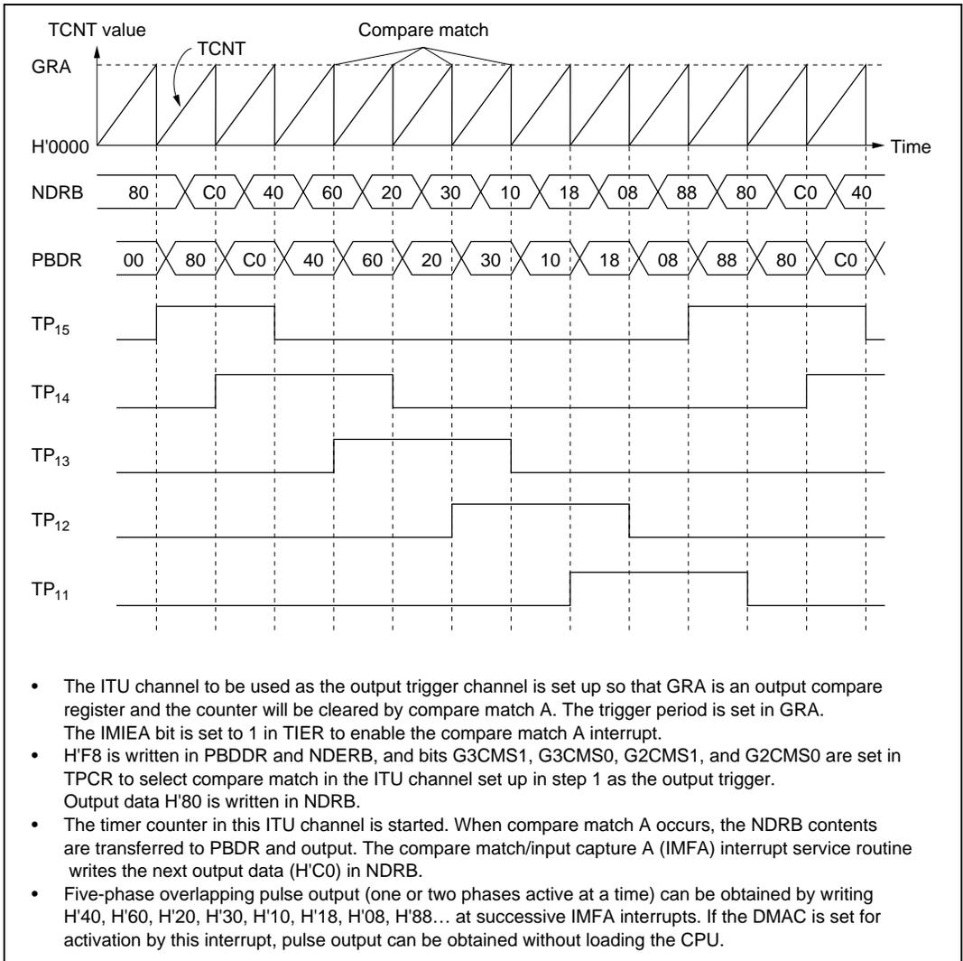
**Figure 11.5 Normal TPC Output Example (Five-Phase Pulse Output)**
