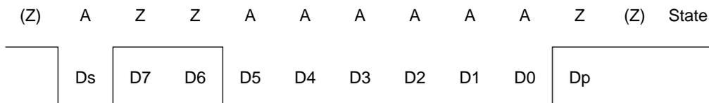
In the inverse convention, state A corresponds to the logic level 1, and state Z to the logic level 0. Characters are transmitted and received MSB-first. In the example above the first character data is H'3F. Following the even parity rule designated for smart cards, the parity bit logic level is 0, corresponding to state Z.
