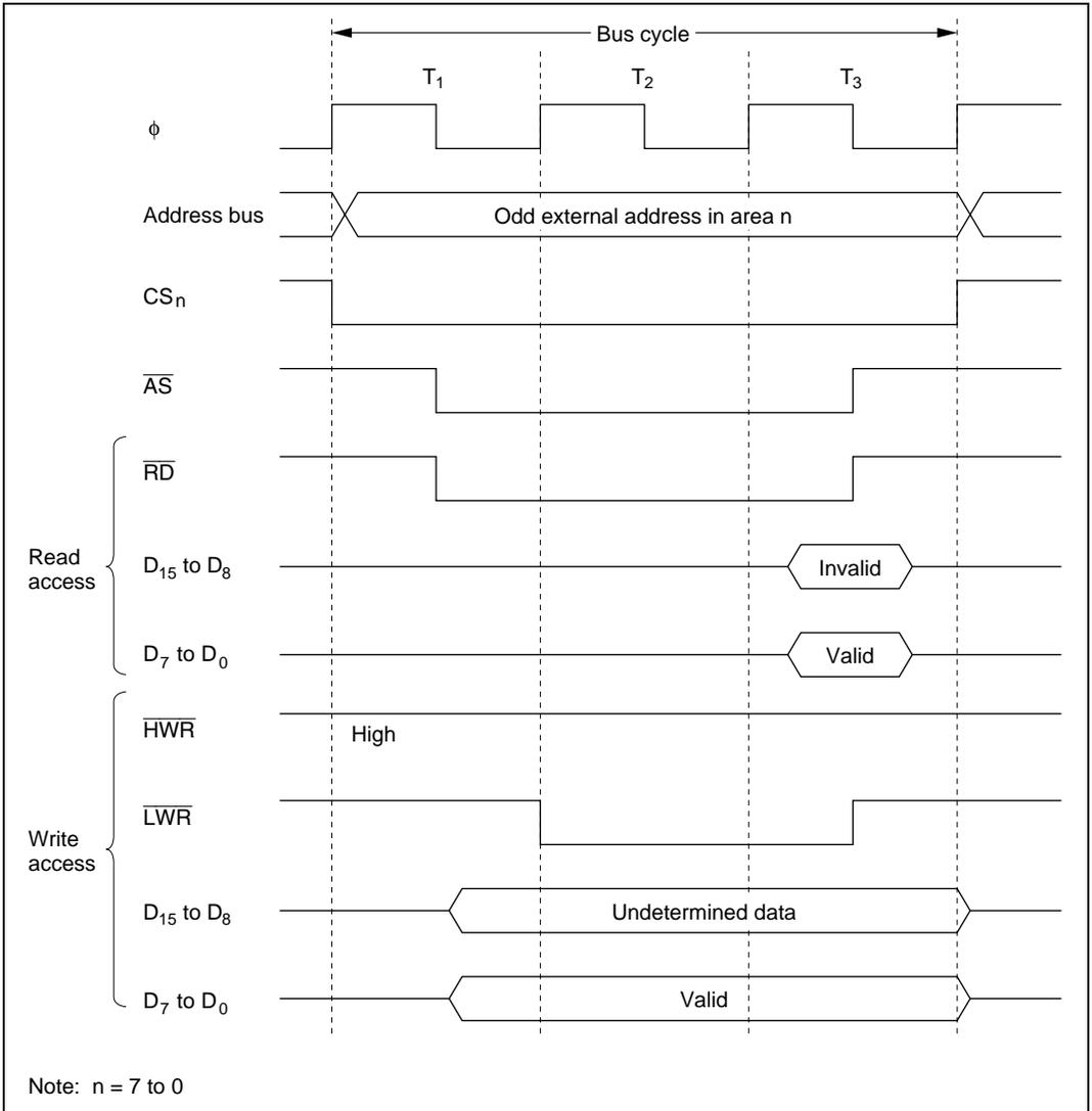
**Figure 6.7 Bus Control Signal Timing for 16-Bit, Three-State-Access Area (2)
