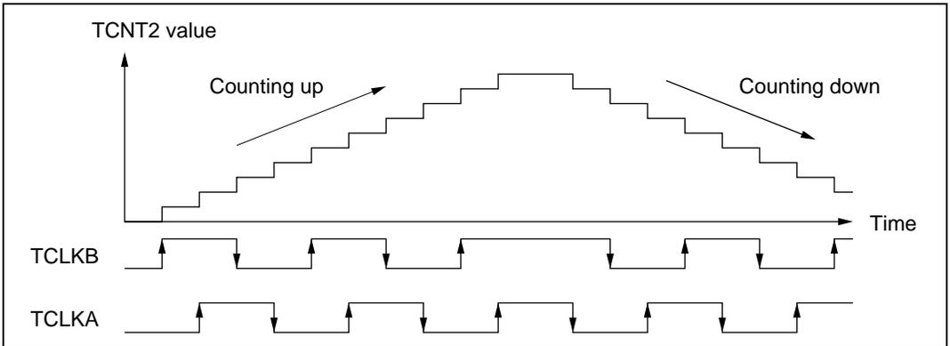
**Figure 10.44 Operation in Phase Counting Mode (Example)**
