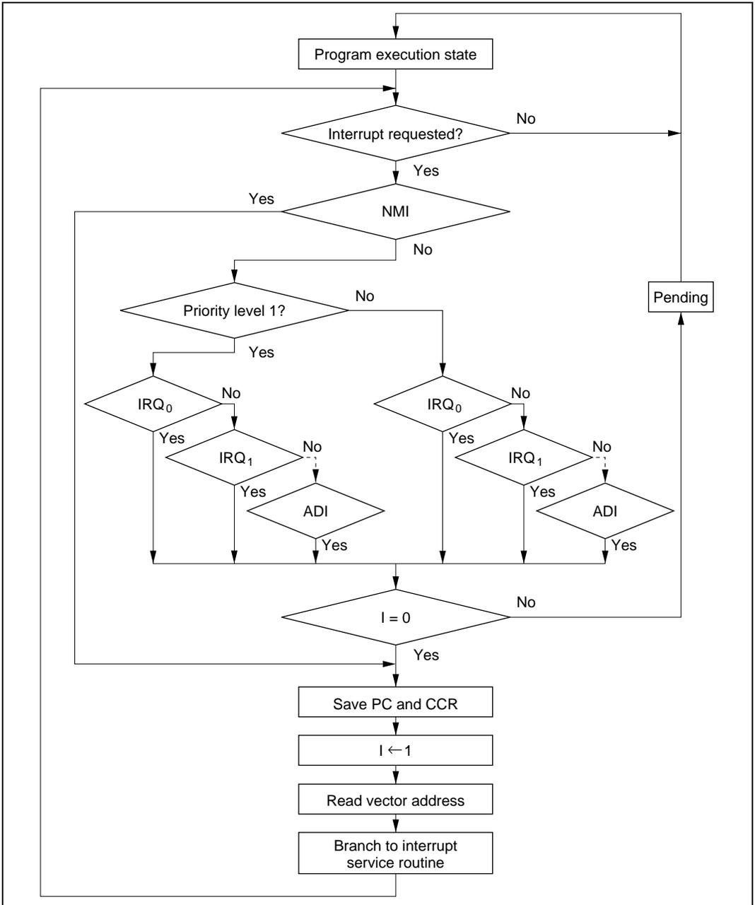
Figure 5.4 Process Up to Interrupt Acceptance when UE = 1
