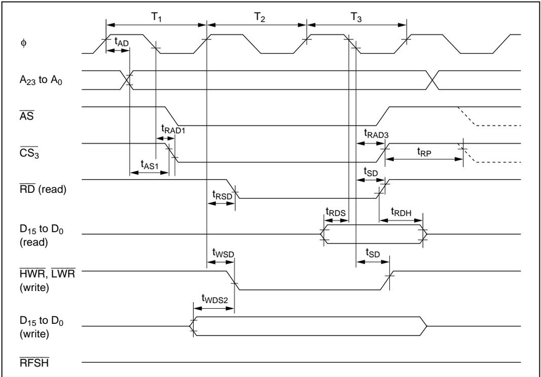
Figure 21.16 PSRAM Bus Timing (Read/Write): Three-State Access
