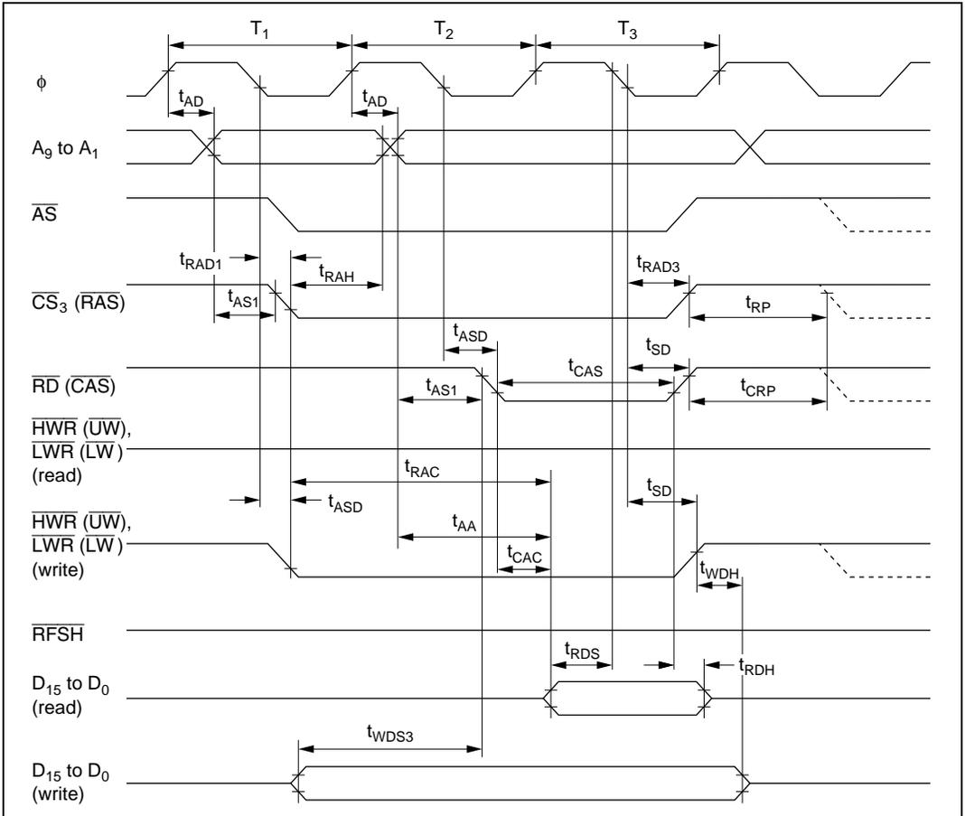
**Figure 21.10 DRAM Bus Timing (Read/Write): Three-State Access**
