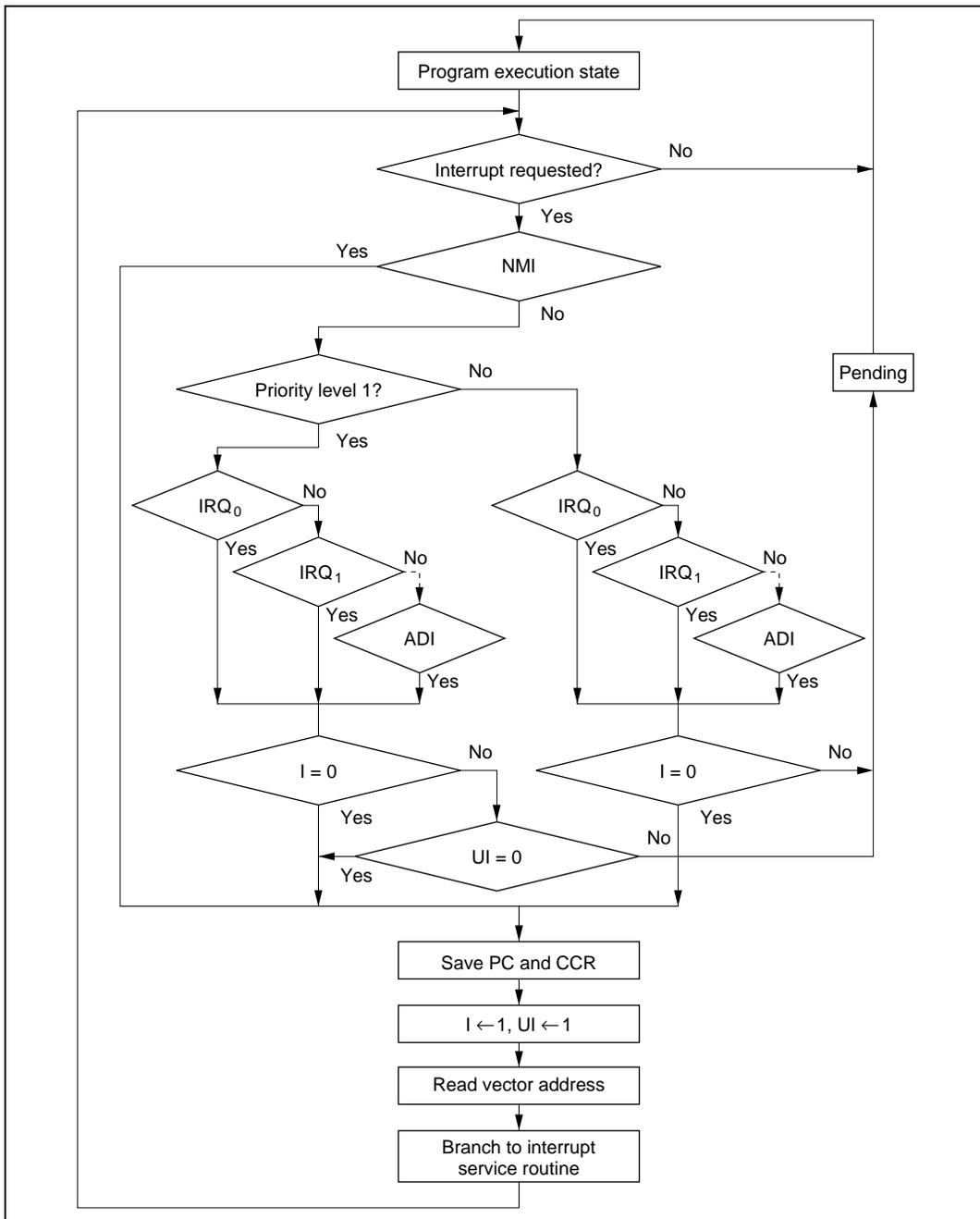
**Figure 5.6 Process Up to Interrupt Acceptance when UE = 0**
