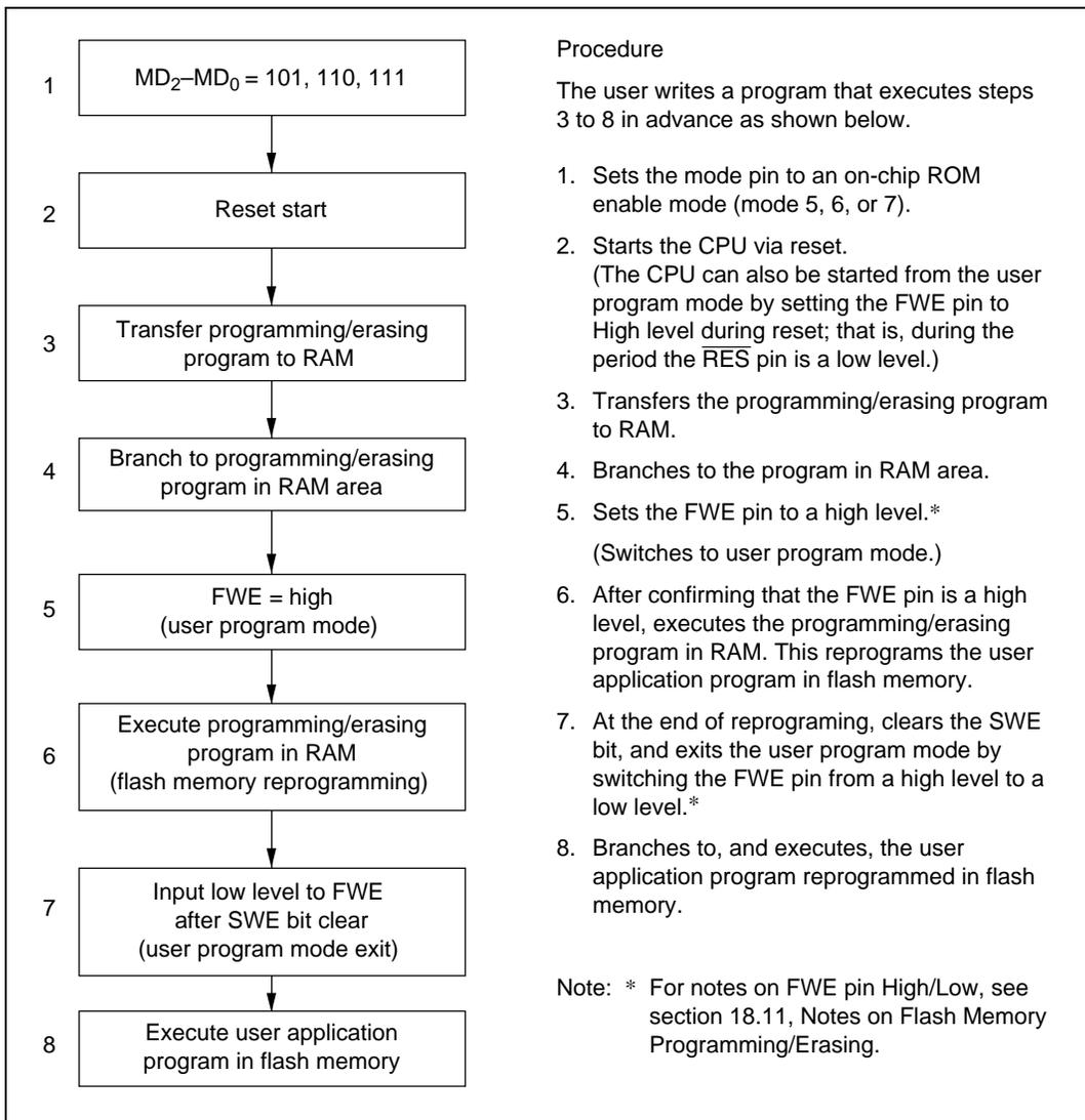
**Figure 18.11 User Program Mode Execution Procedure (Example)**
