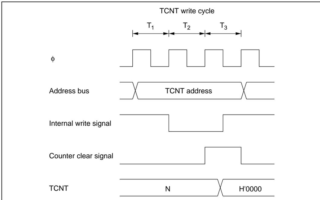
**Figure 10.61** Contention between TCNT Write and Clear
