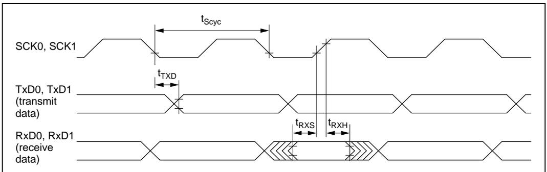
**Figure 21.27 SCI Input/Output Timing in Synchronous Mode**
