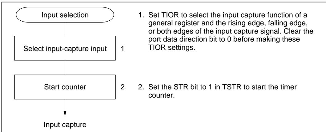
**Figure 10.23 Setup Procedure for Input Capture (Example)**
