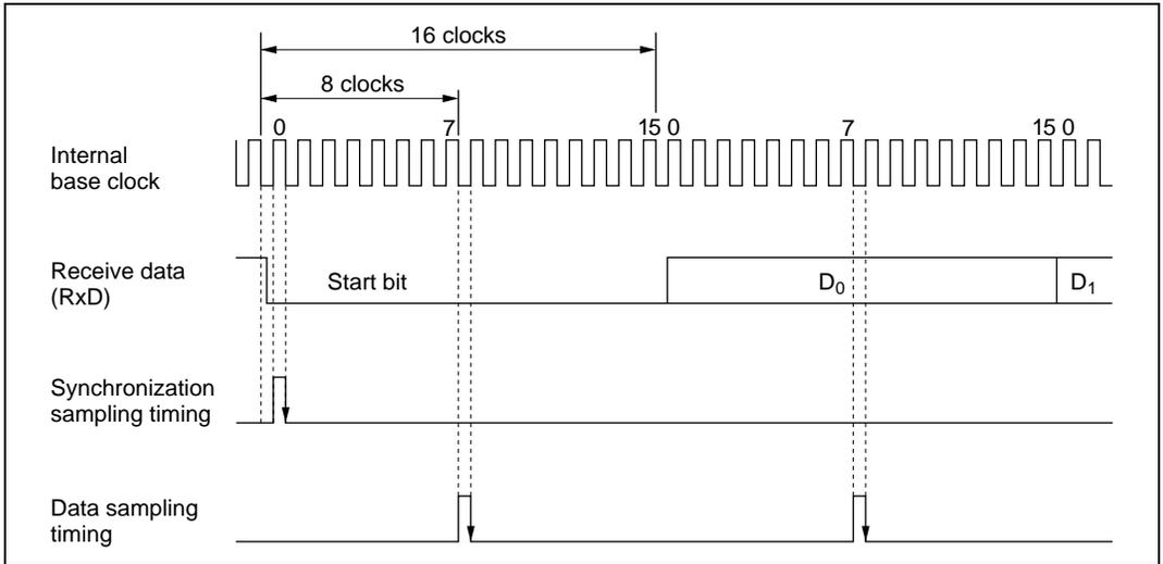
**Figure 13.21 Receive Data Sampling Timing in Asynchronous Mode**
