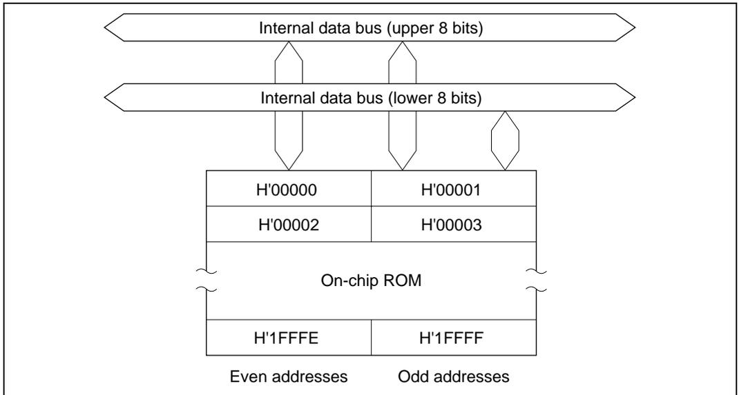
**Figure 18.21 ROM Block Diagram (H8/3048B Mask ROM Version)**
