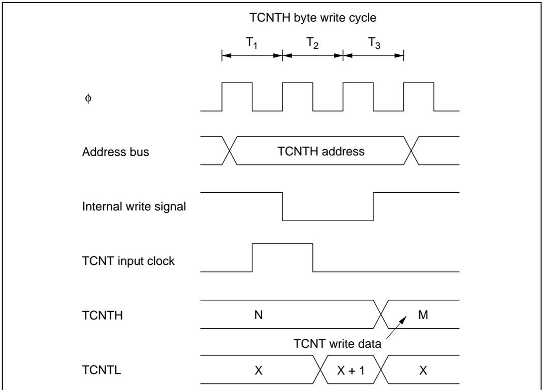
**Figure 10.63** Contention between TCNT Byte Write and Increment
