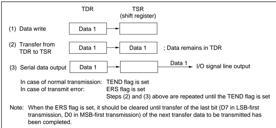
**Figure 14.5 Relation Between Transmit Operation and Internal Registers**
