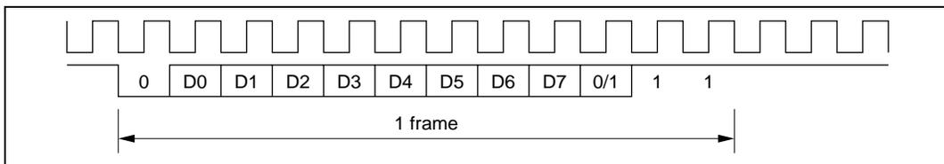
**Figure 13.3 Phase Relationship between Output Clock and Serial Data
