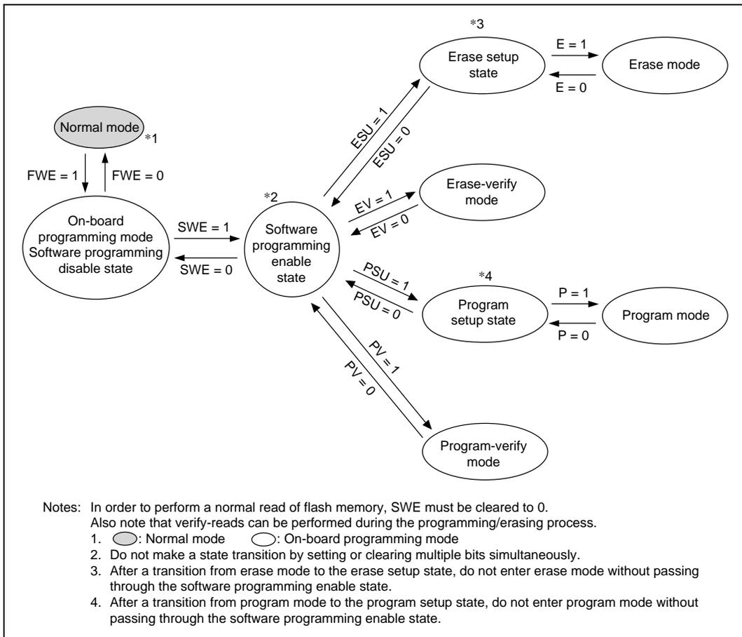
**Figure 18.12 State Transitions Caused by FLMCR1 Bit Settings**
