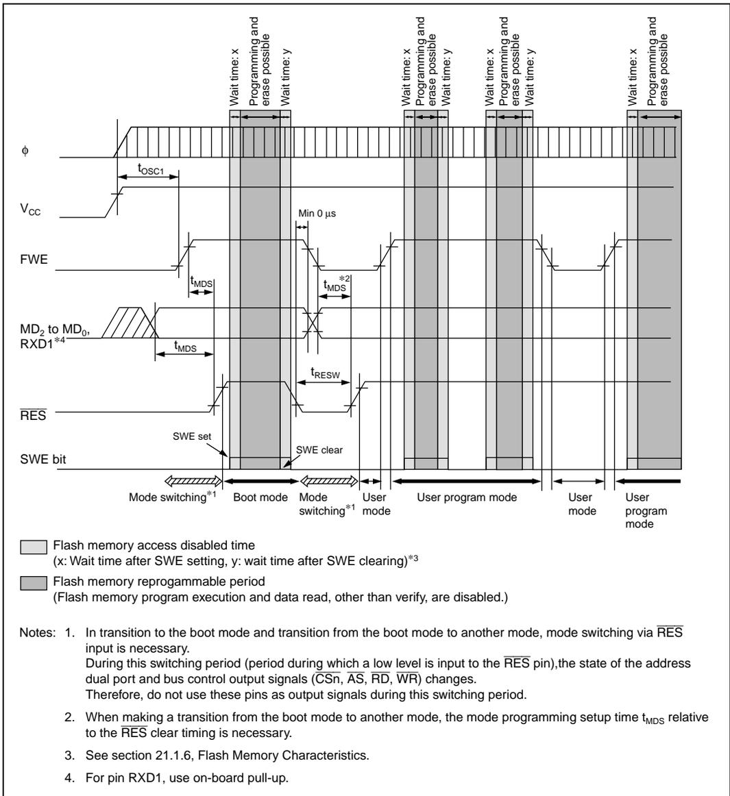
**Figure 18.20 Mode Transition Timing**
