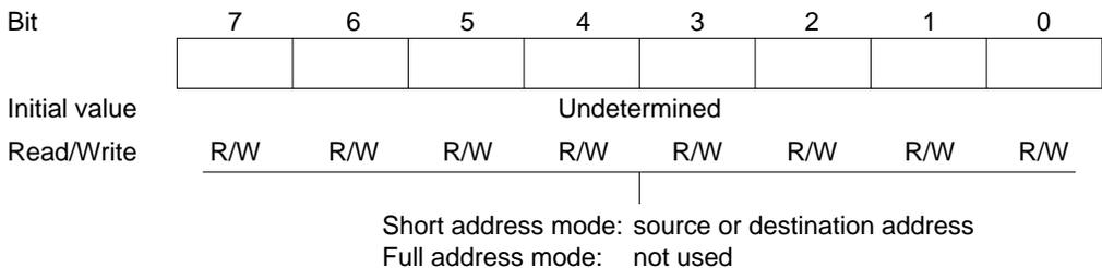
**DTCR0B—Data Transfer Control Register 0B****H'2F****DMAC0**
