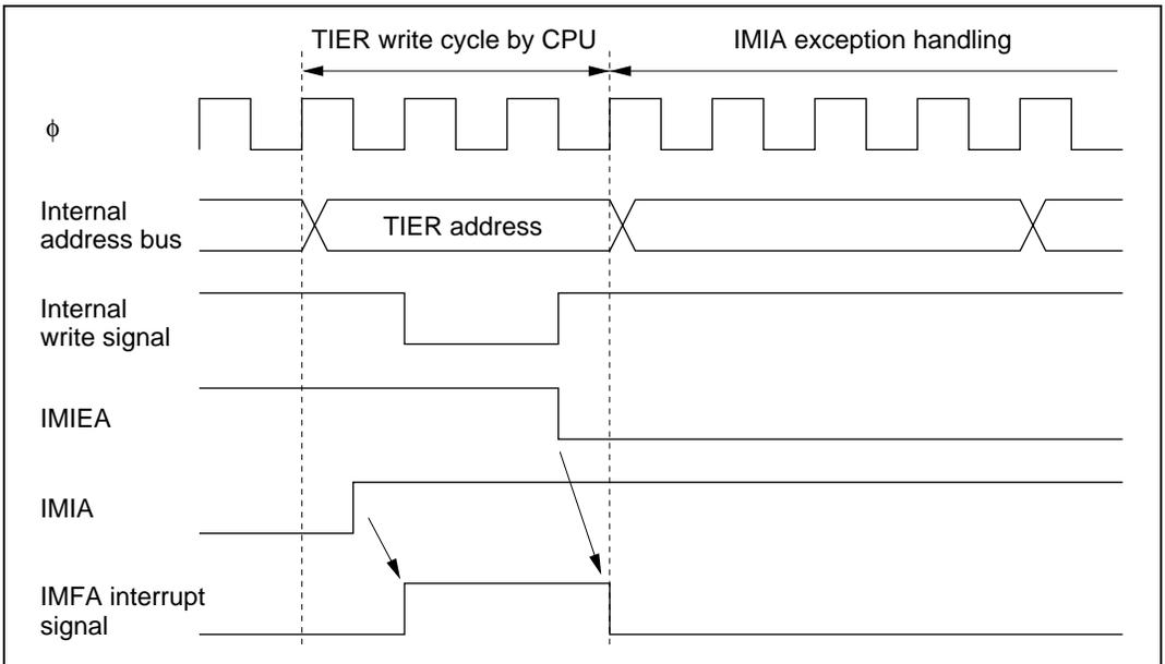
**Figure 5.8 Contention between Interrupt and Interrupt-Disabling Instruction**
