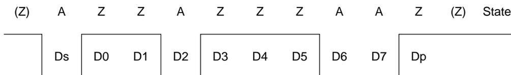
In the direct convention, state Z corresponds to logic level 1, and state A to logic level 0. Characters are transmitted and received LSB-first. In the example above the first character data is H'3B. The parity bit is 1, following the even parity rule designated for smart cards.
