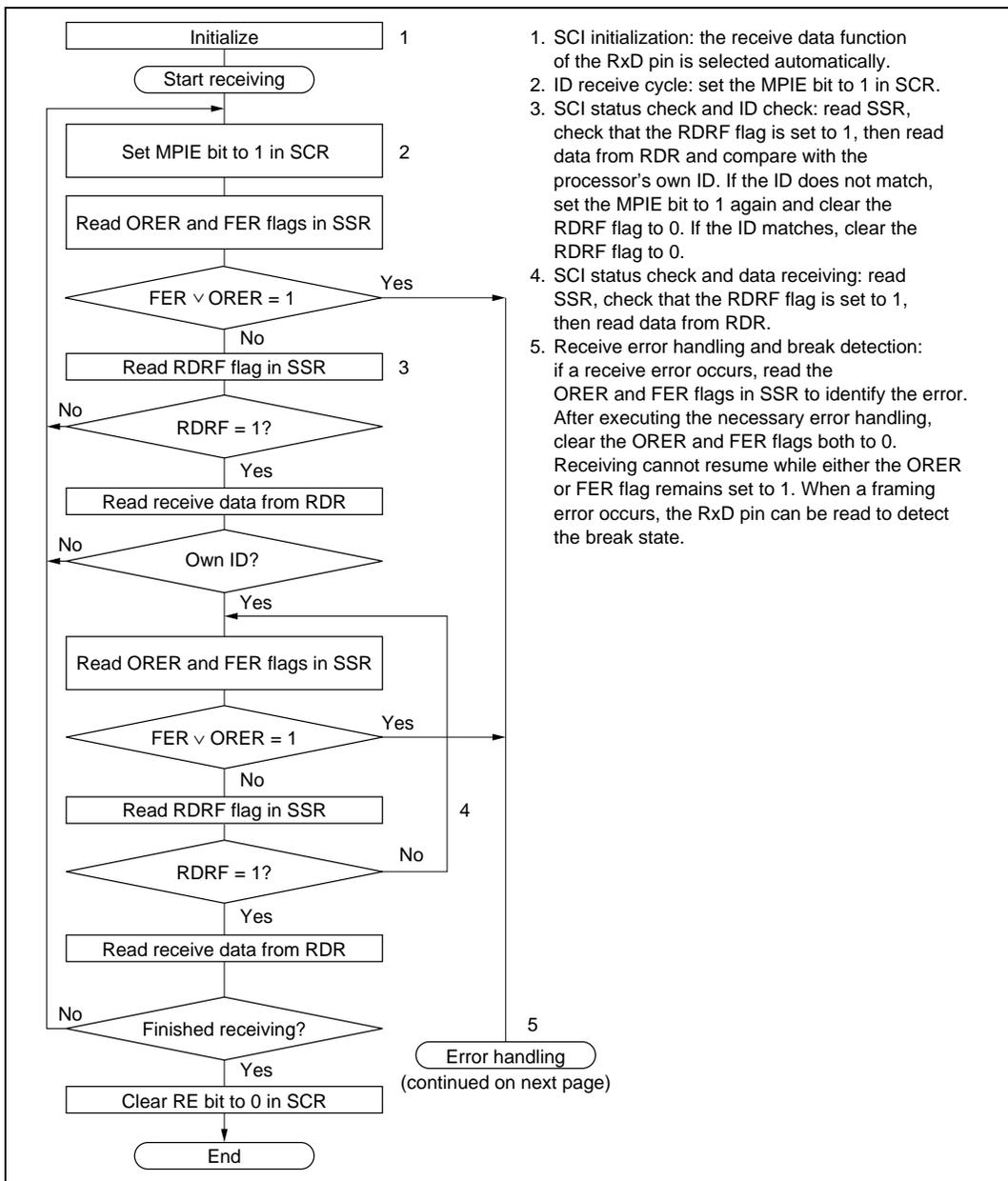
**Figure 13.12 Sample Flowchart for Receiving Multiprocessor Serial Data (1)**
