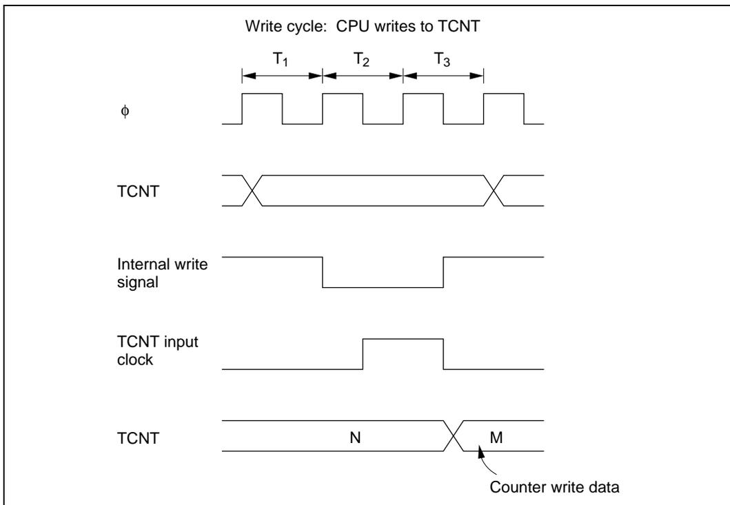
**Figure 12.8 Contention between TCNT Write and Increment**
