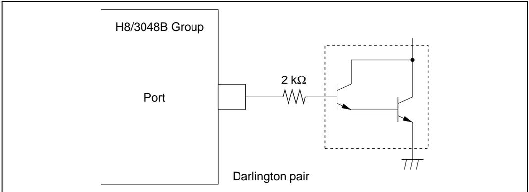
**Figure 21.4 Darlington Pair Drive Circuit (Example)**
