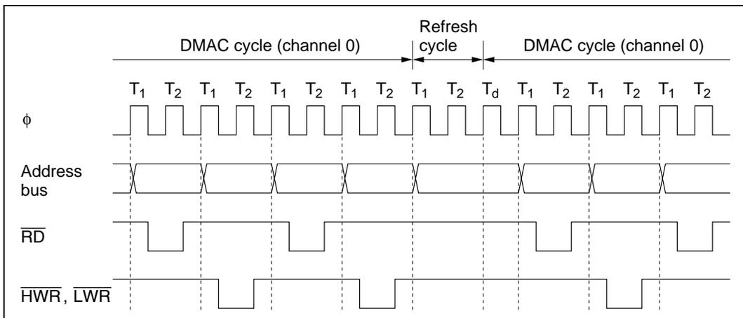
**Figure 8.20 Bus Timing of Refresh Controller and DMAC**
