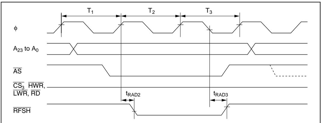
Figure 21.17 PSRAM Bus Timing (Refresh Cycle): Three-State Access
