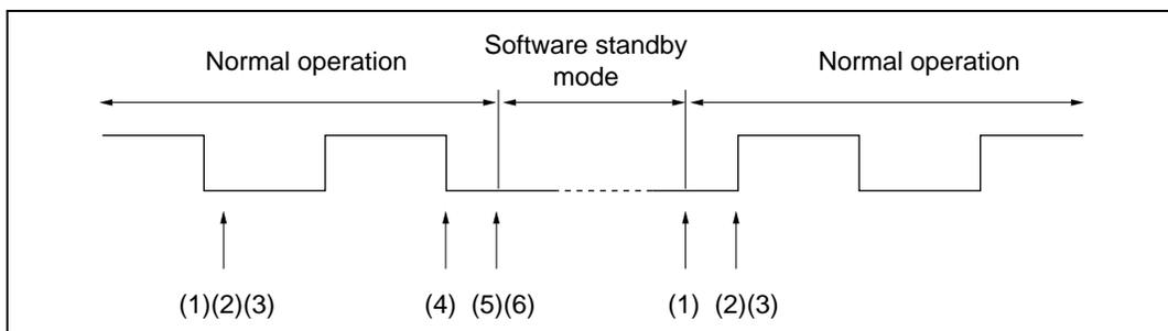
**Figure 14.9 Procedure for Stopping and Restarting the Clock**
