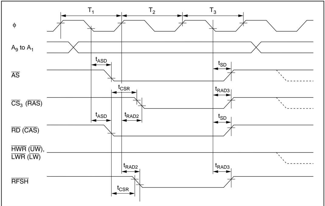
Figure 21.11 DRAM Bus Timing (Refresh Cycle): Three-State Access
