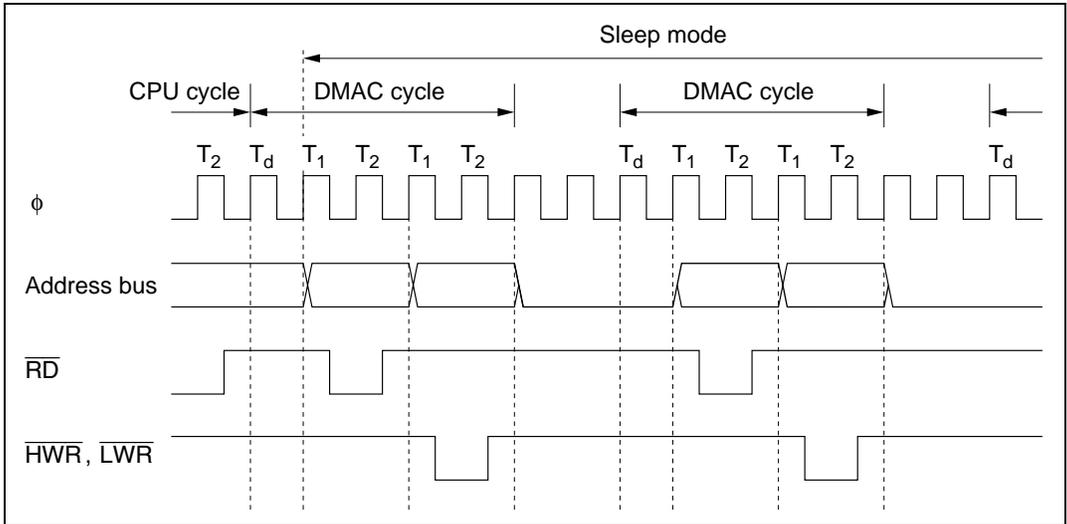
**Figure 8.24 Timing of Cycle-Steal Transfer in Sleep Mode**
