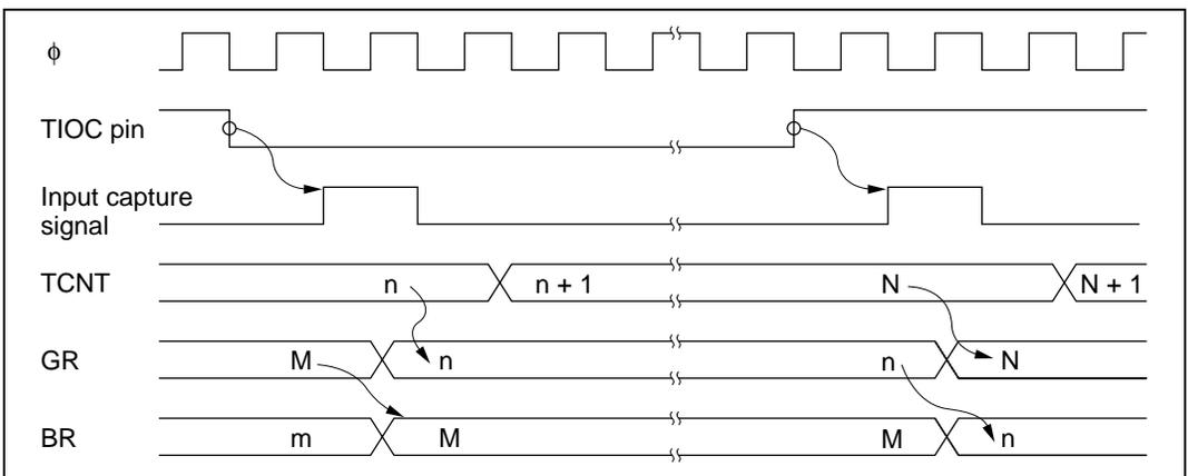
Figure 10.52 Input Capture and Buffer Transfer Timing (Example)
