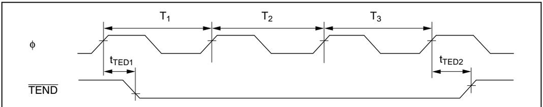
Figure 21.29 DMAC  $\overline{\text{TEND}}$  Output Timing for 3 State Access
