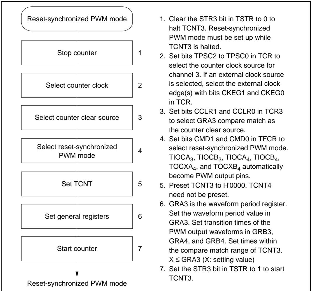
**Figure 10.31 Setup Procedure for Reset-Synchronized PWM Mode (Example)**
