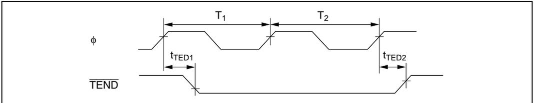
Figure 21.28 DMAC  $\overline{\text{TEND}}$  Output Timing for 2 State Access
