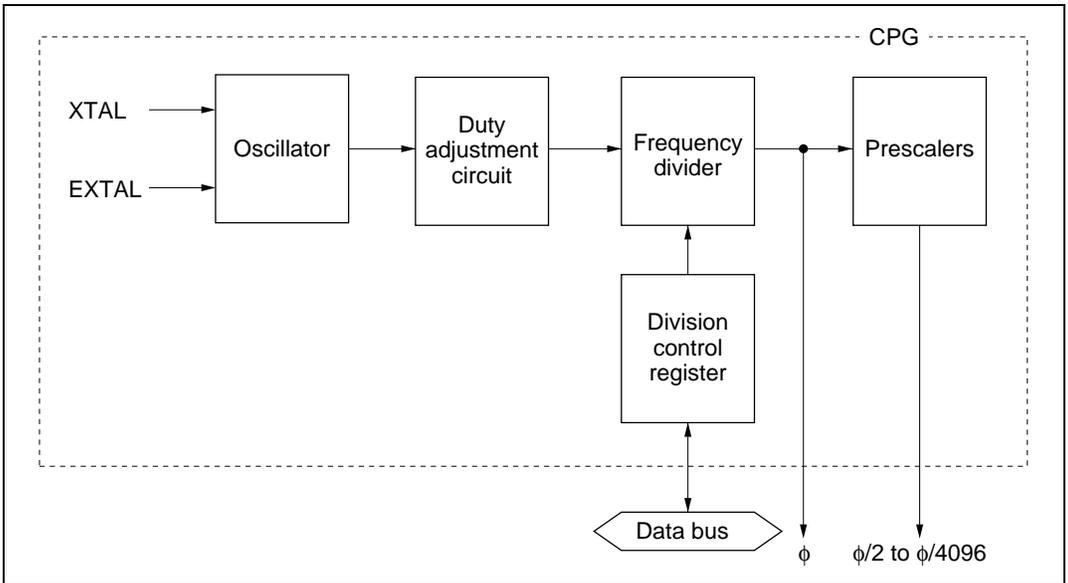
**Figure 19.1 Block Diagram of Clock Pulse Generator**
