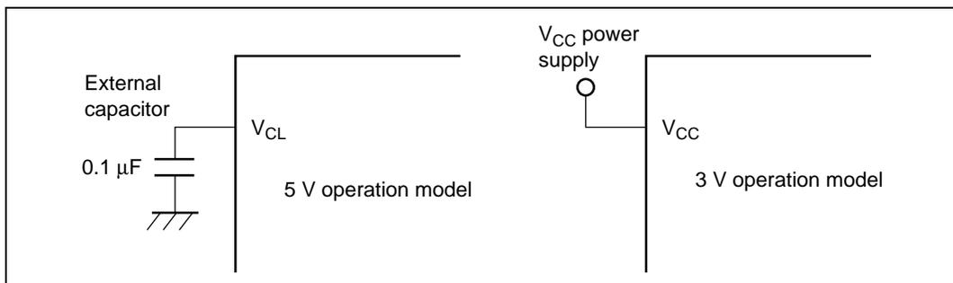
**Figure 1.5** Difference between 5 V and 3 V Operation Models
