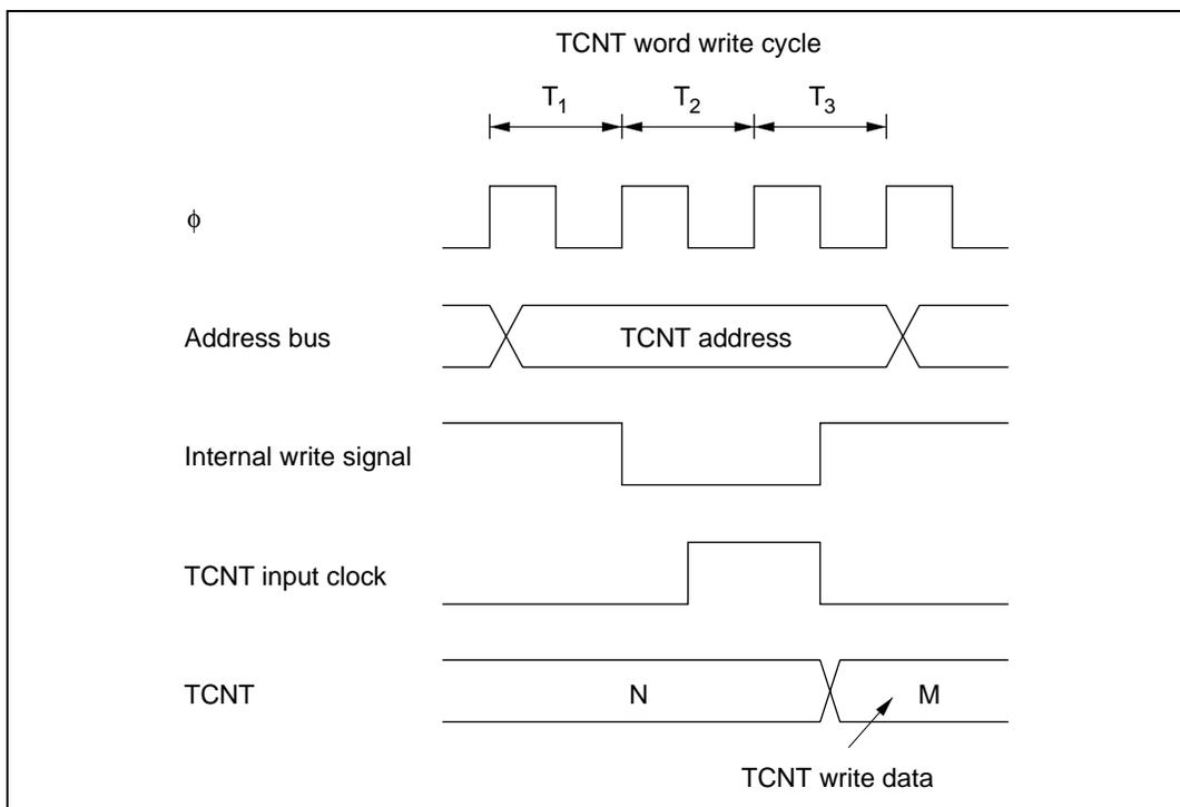
**Figure 10.62** Contention between TCNT Word Write and Increment
