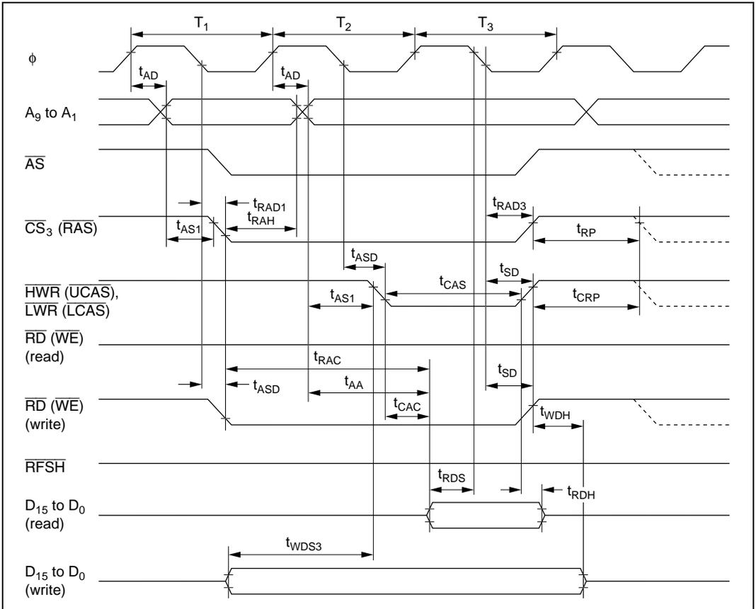
**Figure 21.13 DRAM Bus Timing (Read/Write): Three-State Access**
