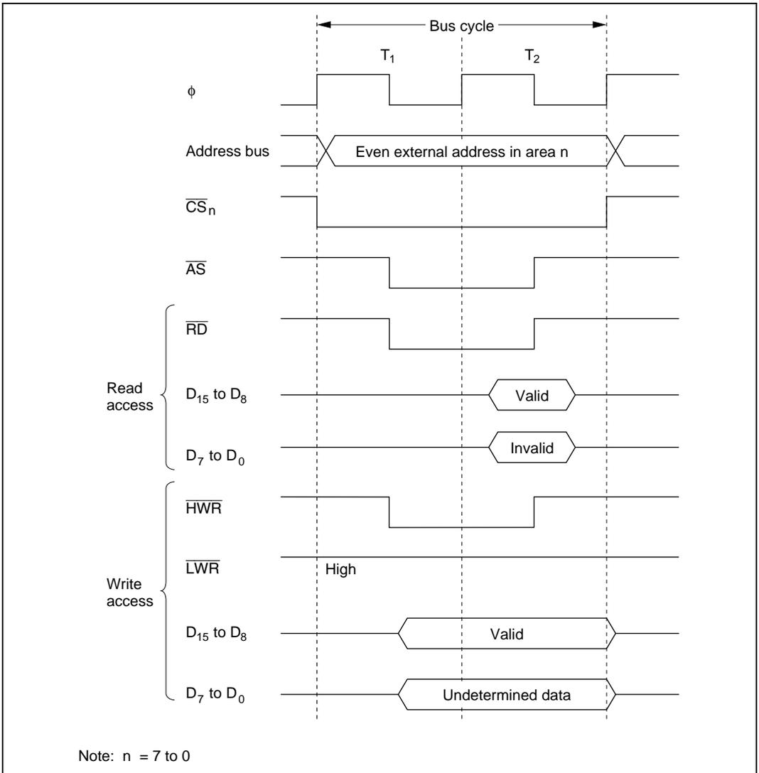
**Figure 6.9 Bus Control Signal Timing for 16-Bit, Two-State-Access Area (1)**
