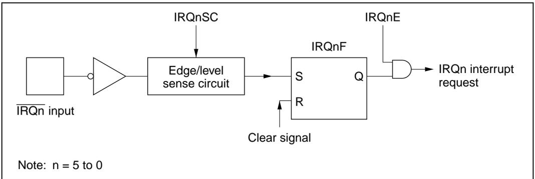
**Figure 5.2 Block Diagram of Interrupts  $\text{IRQ}_0$  to  $\text{IRQ}_5$**
