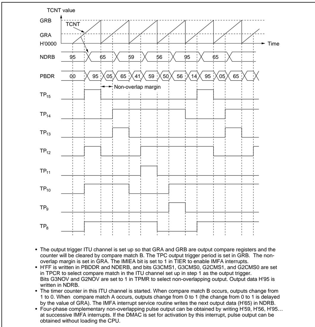
**Figure 11.7 Non-Overlapping TPC Output Example
