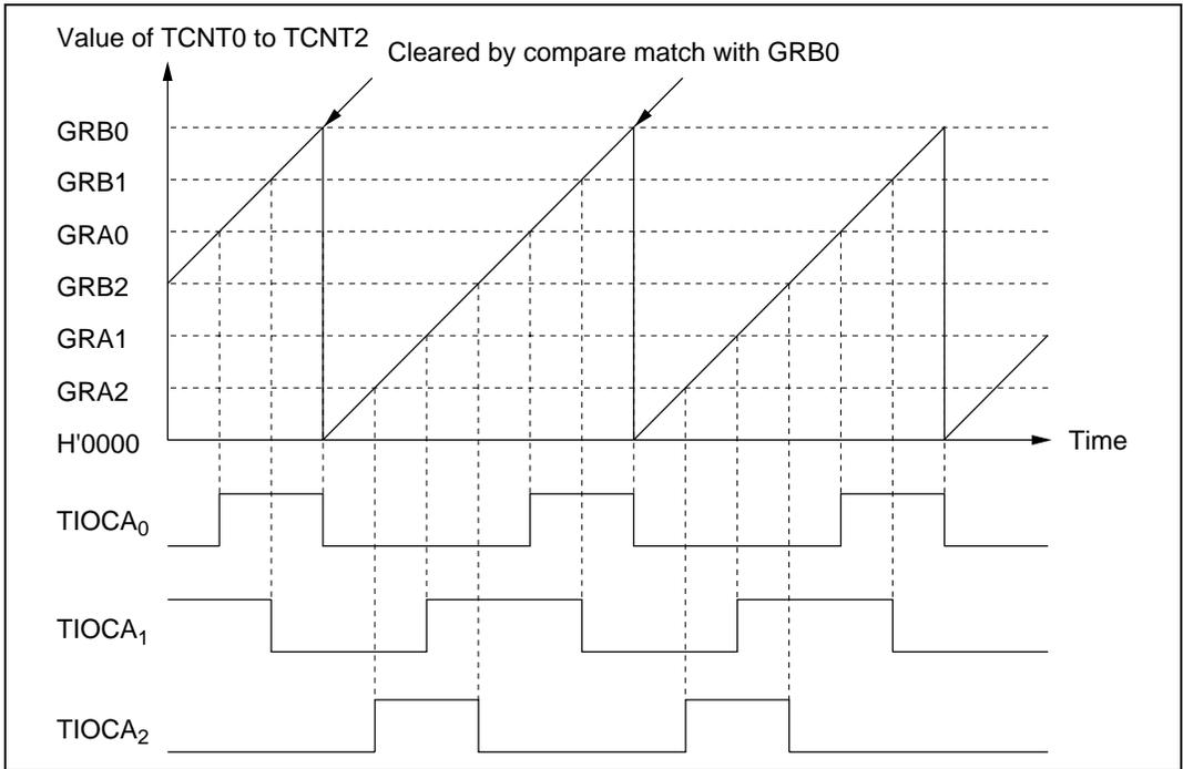
**Figure 10.27 Synchronization (Example)**
