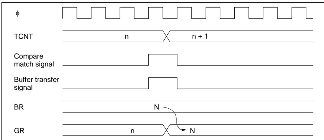
**Figure 10.50 Compare Match and Buffer Transfer Timing (Example)**
