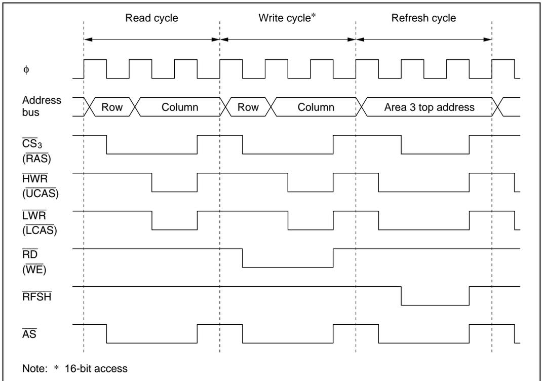
**Figure 7.5(2) DRAM Control Signal Output Timing (2CAS Mode)**
