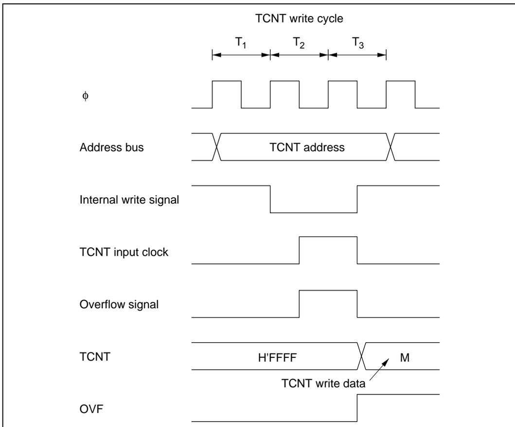
**Figure 10.65** Contention between TCNT Write and Overflow
