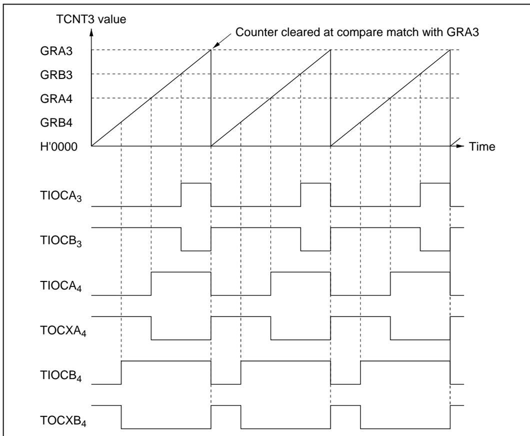
**Figure 10.32 Operation in Reset-Synchronized PWM Mode (Example)**
