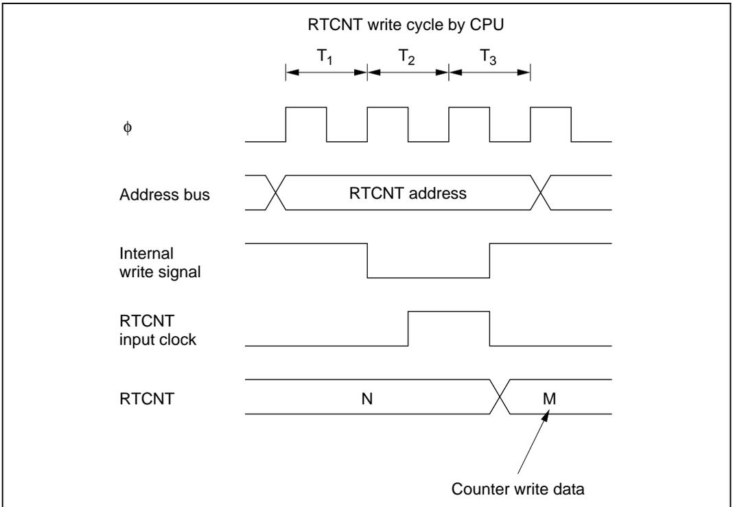
**Figure 7.21 Contention between RTCNT Write and Increment**
