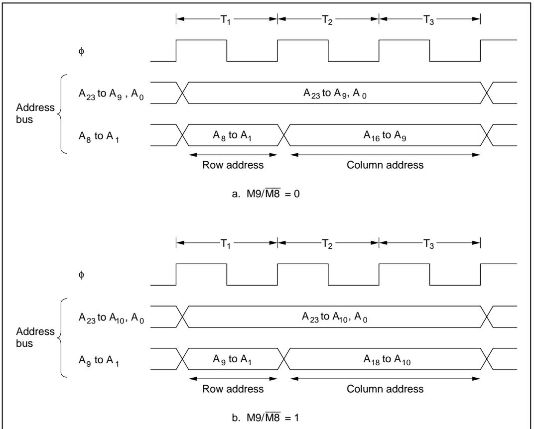
Figure 7.4 Multiplexed Address Output (Example without Wait States)
