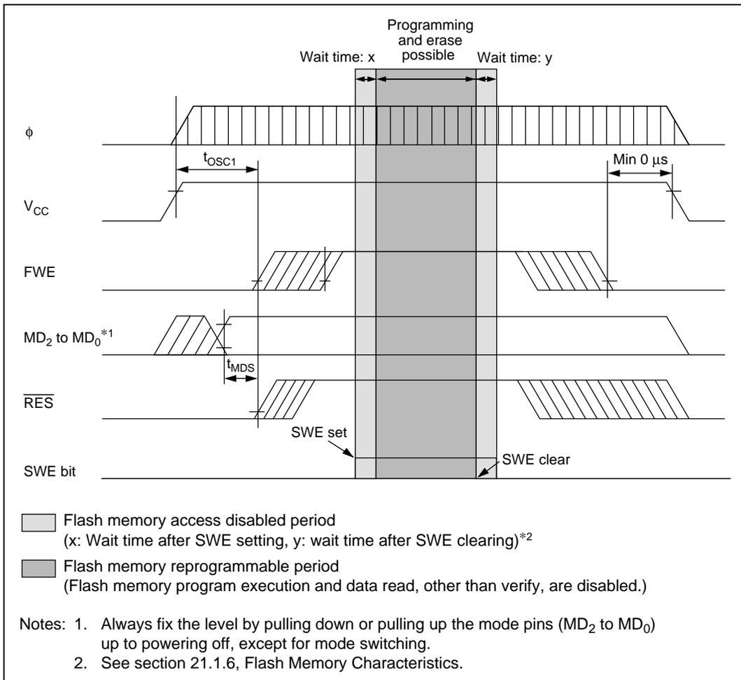
**Figure 18.19 Powering On/Off Timing (User Program Mode)**
