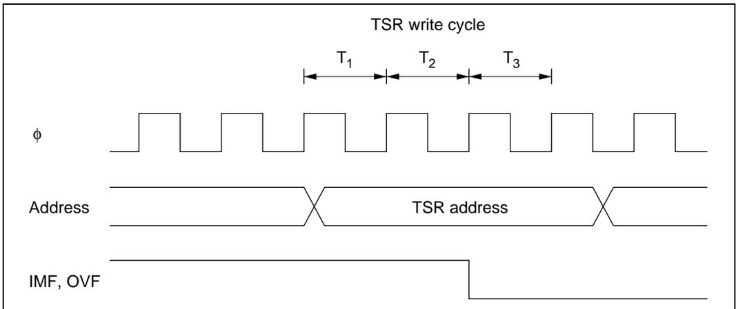
**Figure 10.60 Timing of Clearing of Status Flags**
