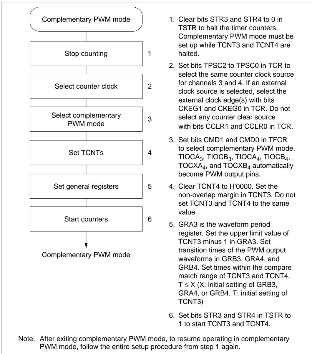
**Figure 10.33 Setup Procedure for Complementary PWM Mode (Example)**
