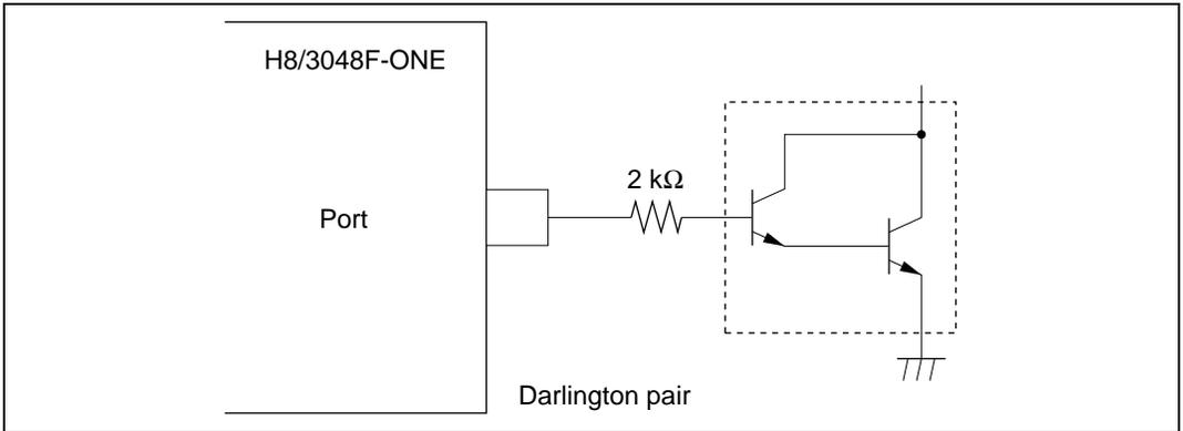
**Figure 21.1 Darlington Pair Drive Circuit (Example)**
