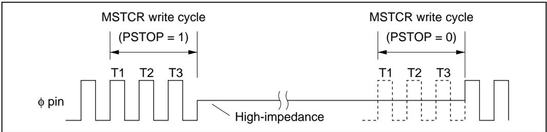
**Figure 20.3 Starting and Stopping of System Clock Output**
