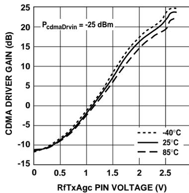
Figure 8. CDMA Driver Gain vs. V(RfTxAgc) and Temperature.
