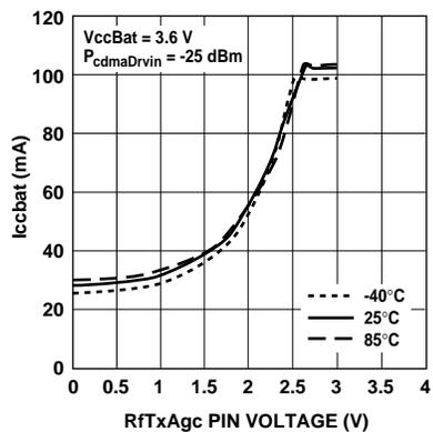
Figure 7. CDMA Driver IccBat vs. V(RfTxAgc) and Temperature.
