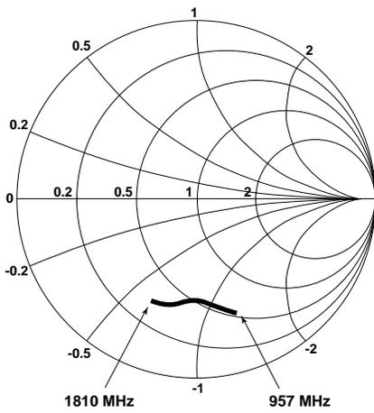
**Figure 22. LO Port Input Impedance vs. Frequency.**
