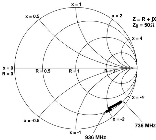
**Figure 24. ampsMixOut Output Impedance vs. Frequency.**
