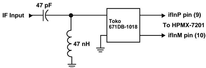
Figure 32. Test Circuit for Single-ended 50Ω IF Operation.
