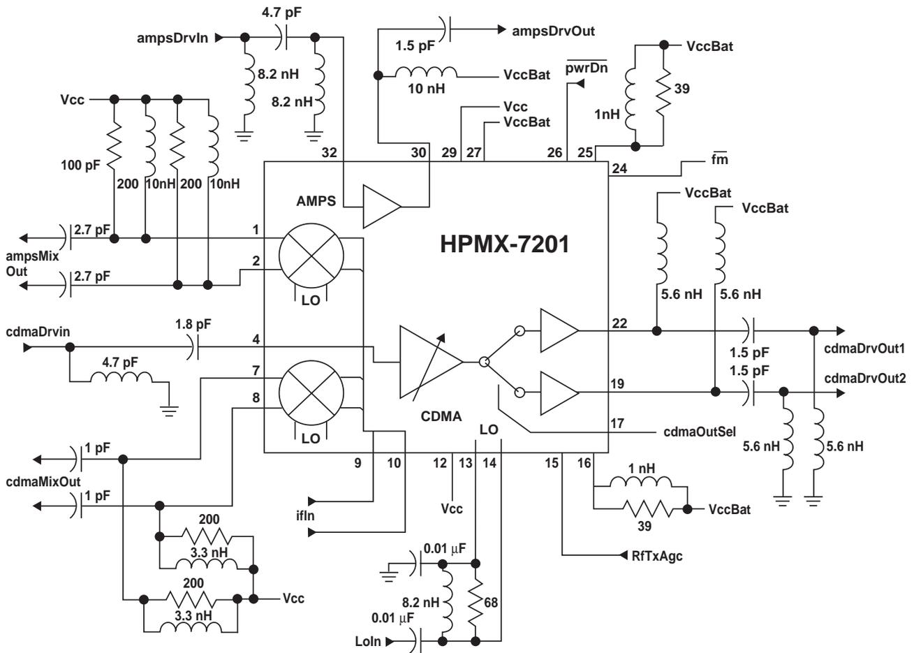
Figure 31. Example Reference Circuit for the HPMX-7201.
