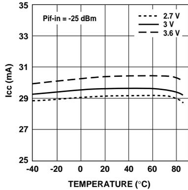
Figure 1. CDMA Upconverter Icc vs. Vcc and Temperature.
