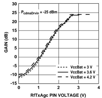
Figure 9. CDMA Driver Gain vs. V(RfTxAgc) and VccBat.
