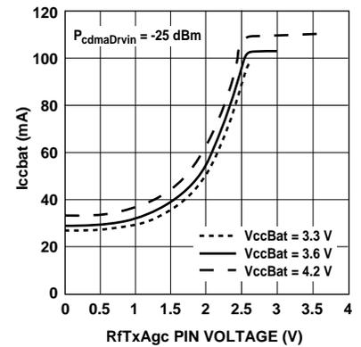
Figure 6. CDMA Driver Iccbat vs. V(RfTxAgc) and VccBat.
