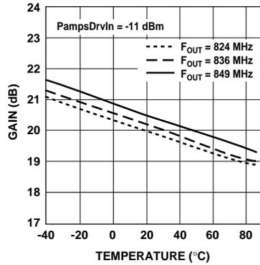
**Figure 20. AMPS Driver Gain vs. Temperature and Frequency.**
