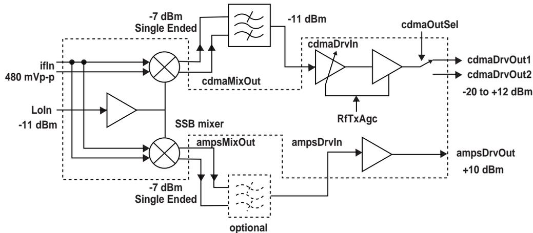
Figure 33. Expected Power and Voltage Levels.
