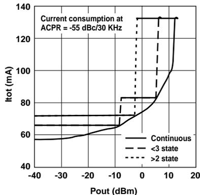
**Figure 36: HPMX-7201 Total Current Consumption vs. Output Power and Control Method.**
