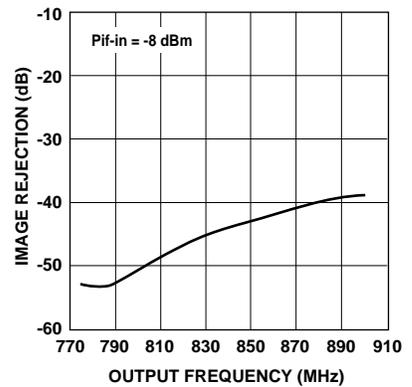
**Figure 18. AMPS Upconverter Image Rejection vs. Output Frequency.**
