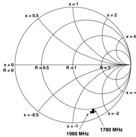
**Figure 23. cdmaMixOut Output Impedance vs. Frequency.**
