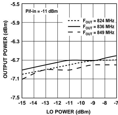
**Figure 17. AMPS Upconverter Output Power vs. LO Power and Frequency.**
