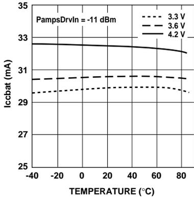
**Figure 19. AMPS Driver IccBat vs. Temperature and VccBat.**
