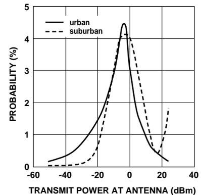
Figure 34: Probability Distribution of Mobile Transmit Power.
