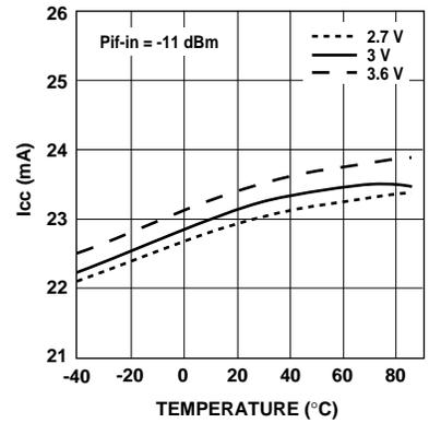
**Figure 15. AMPS Upconverter Icc vs. Temperature and Vcc.**
