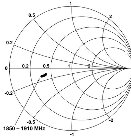
**Figure 25. cdmaDrvIn Input Impedance vs. Frequency.**
