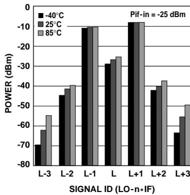
Figure 5. CDMA Upconverter Output Spectrum vs. Temperature.
