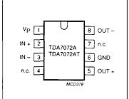
Fig.2 Pinning diagram.
