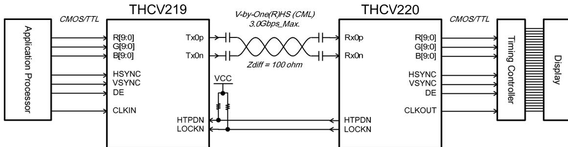
Example for CMOS/TTL to CMOS/TTL
