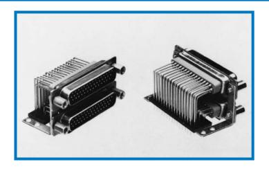
High Density Dual Port Series connectors utilize two high density connectors vertically stacked and assembled into a single connector unit, which permits saving of panel and printed board space, and decreases final assembly costs.
