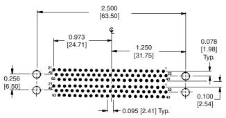
Mounting hole must move 0.020 [0.51] opposite direction of the arrow for use of unriveted mounting brackets with connectors.
