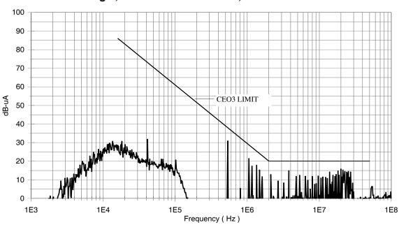
Fig 1, Conducted Emissions, Positive Lead
