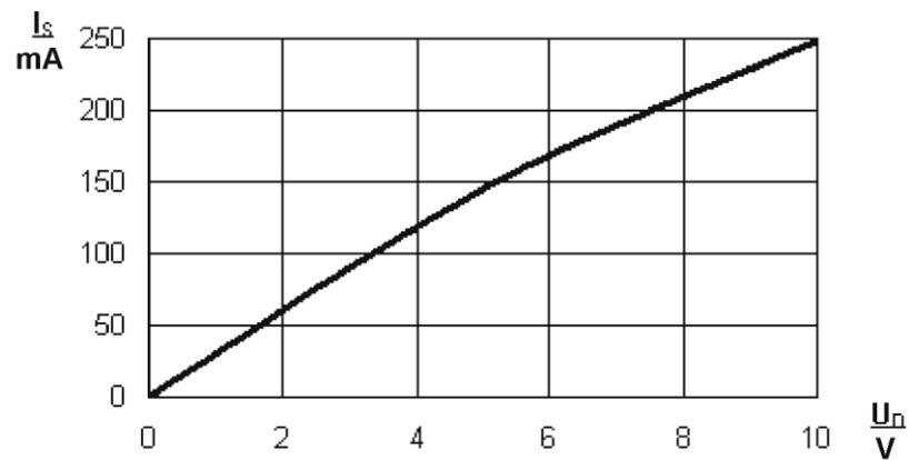
Fig. 4 – DRAIN consumption current  $I_s$  vs DRAIN supply voltage  $V_D$
