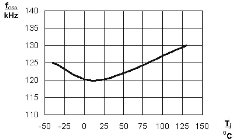
Fig. 3 – Average operating frequency  $f_{osc}$  vs. temperature  $T_j$
