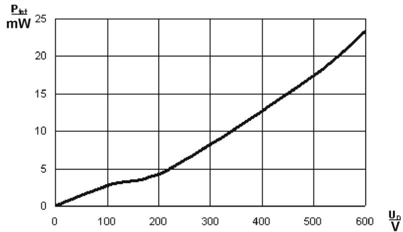
Fig. 5 –Power dissipation  $P_{tot}$  vs DRAIN supply voltage  $V_D$
