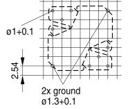
Hole arrangement View in mounting direction
