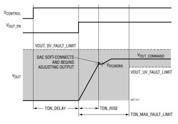
Figure 17. Typical On Sequence Using Control Pin
