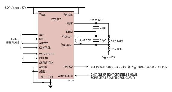
Figure 29. Sensing Negative Voltages
