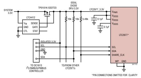
NOTE: DC1613 CONTROLLER  $l^2C$  CONNECTIONS ARE OPTO-ISOLATED ISOLATED 3.3V FROM CONTROLLER CAN BE BACK DRIVEN AND WILL ONLY DRAW <  $10\mu A$  ISOLATED 3.3V CURRENT LIMIT = 100mA
