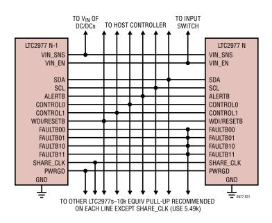
Figure 21. Typical Connections Between Multiple LTC2977s
