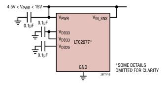
Figure 15. Powering LT2977 Directly from an Intermediate Bus
