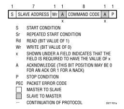
Figure 1a. PMBus Packet Protocol Diagram Element Key
