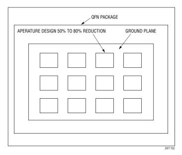
Figure 32. Suggested Screen Pattern for Die Attach Pad
