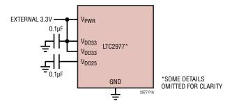
Figure 16. Powering LTC2977 from External 3.3V Supply
