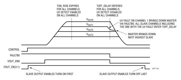
Figure 13c. Fault on Channel 1 Tracking All Supplies Down
