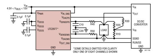
Figure 28. Antialiasing Filter on V<sub>SENSE</sub> Lines
