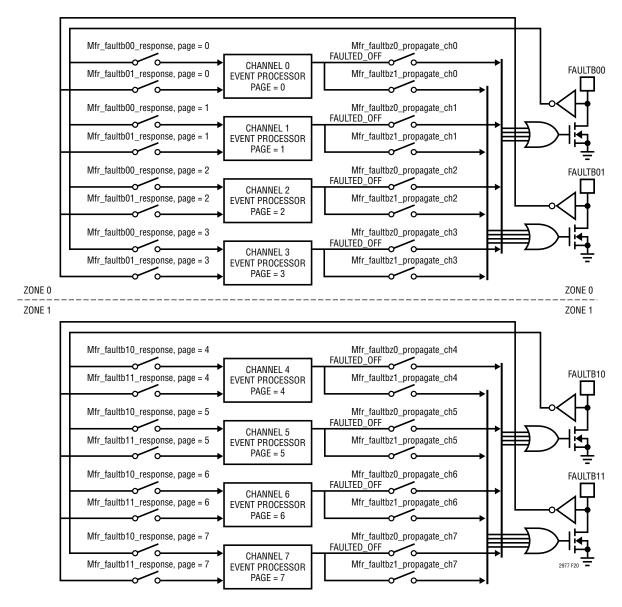
Figure 20. Channel Fault Management Block Diagram
