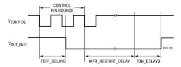
Figure 18. Off Sequence with Automatic Restart
