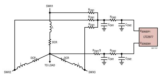
Figure 27. Multiphase DCR Current Sensing Circuits
