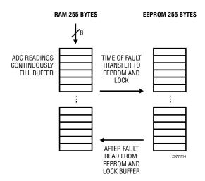
Figure 14. Fault Log Conceptual Diagram
