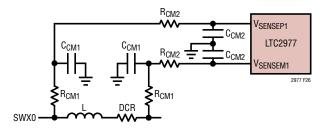
Figure 26. Inductor DCR Current Sensing Circuits
