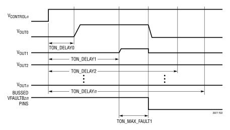
Figure 22. Aborted On Sequence Due to Channel 1 Short
