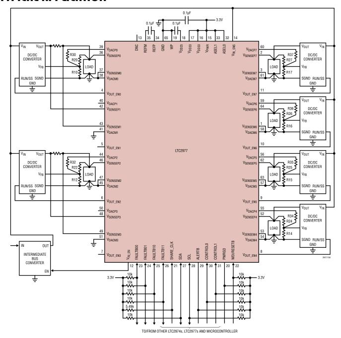
Figure 34. LTC2977 Application Circuit with 3.3V Chip Power
