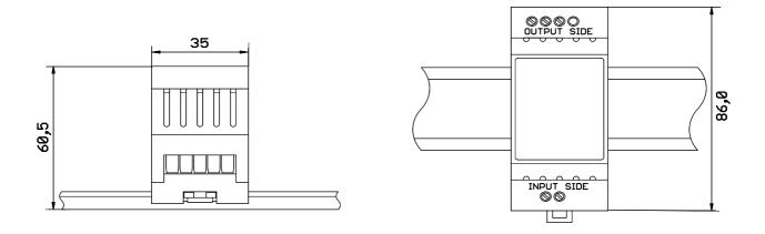
Case material is for the top cover (Lexan), lower case (Noryl). Class UL94V0 Top cover includes ventilating louvers for cooling by air convection
