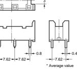
PCB Mounting Holes (BOTTOM VIEW)
