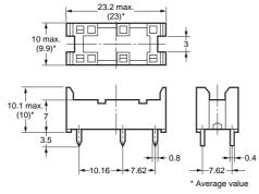
PCB Mounting Holes (BOTTOM VIEW)
