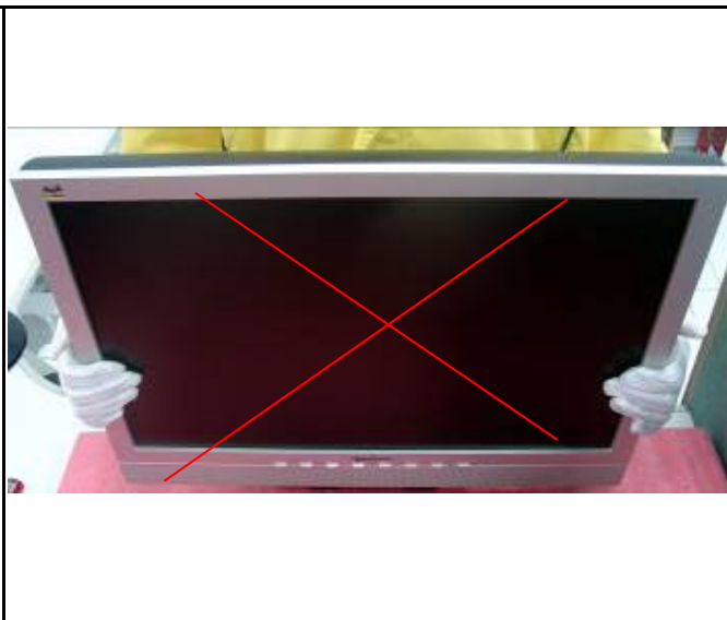
when assemble&disassembly bezel
