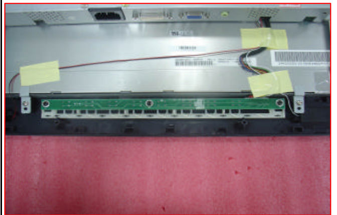
pull out button/b cable from button/b connector(12)
