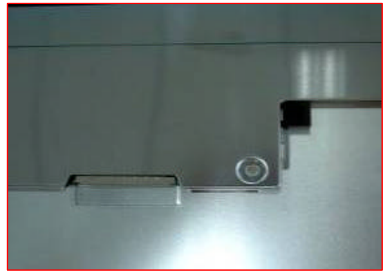
tear off mylar and rubber(16)
