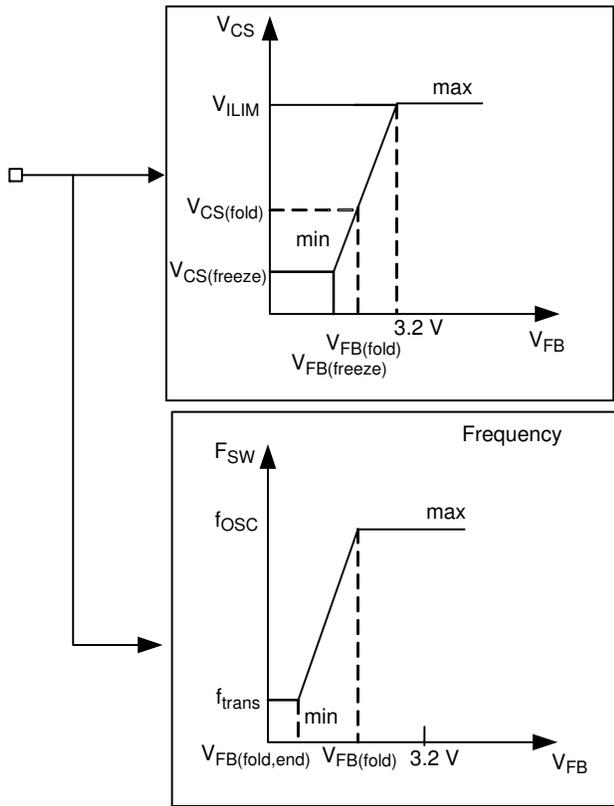
Figure 6. Frequency Foldback Architecture
