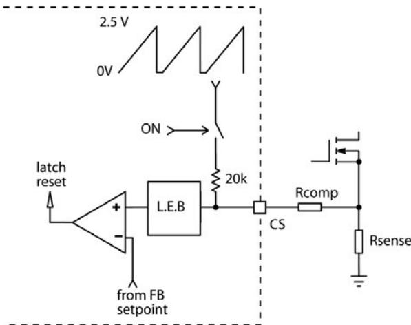
**Figure 9. Internal Adjustable Ramp Compensation Architecture**
