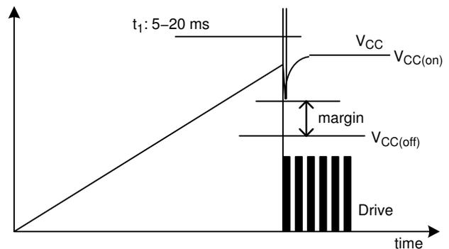
Figure 4. Startup Process for NCP1136
