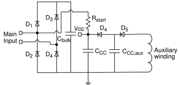
**Figure 5. Startup Circuit for NCP1136 (half-wave connection), Considering Light Load Condition**
