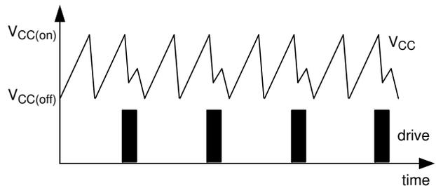
Figure 8. Auto-Recovery Double Hiccup Sequence
