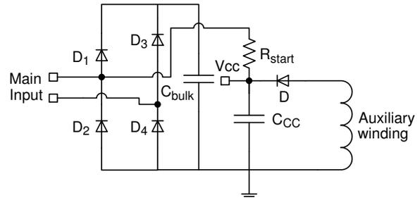
Figure 3. Startup Circuit for NCP1136 (half-wave connection)
