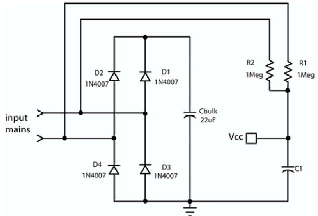
Figure 7. The Full-wave Connection Ensures Latch Current Continuity as Well as a X2-Discharge Path
