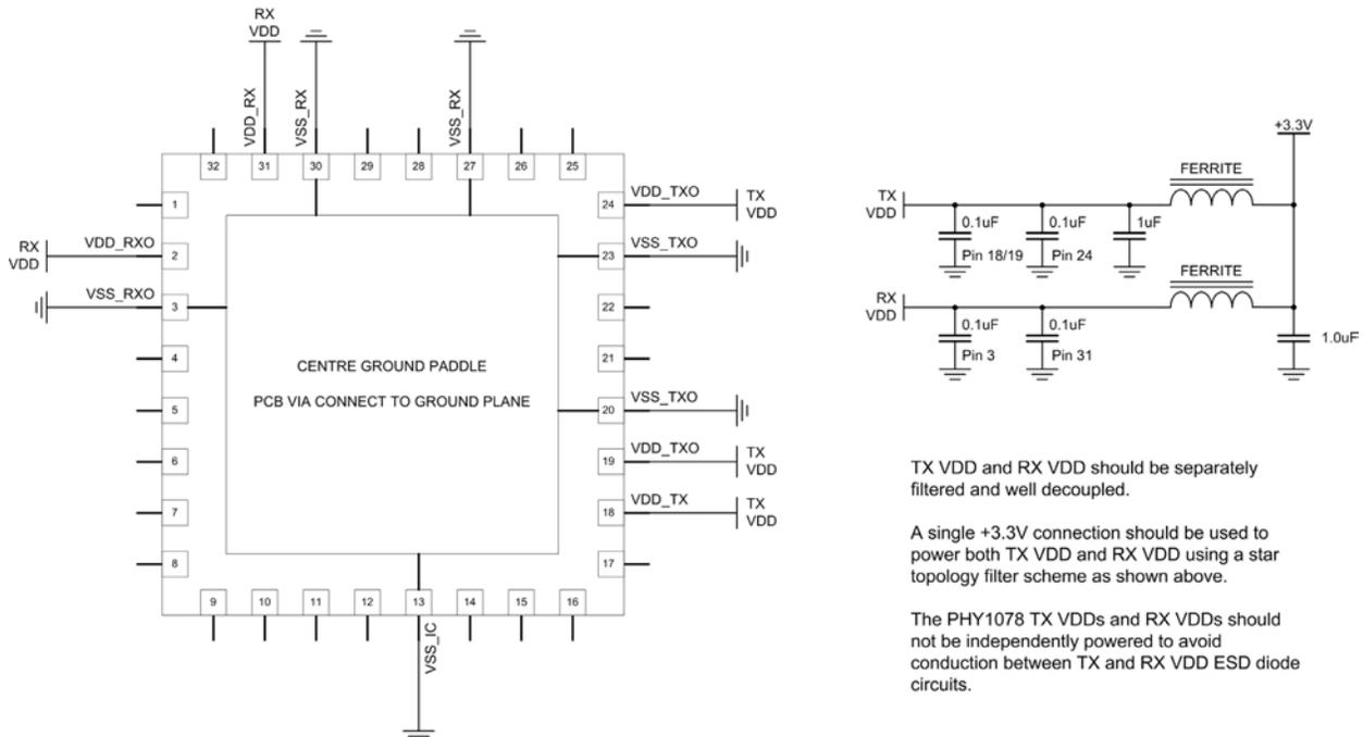
Figure 33 – Recommended power supply connections and filtering.
