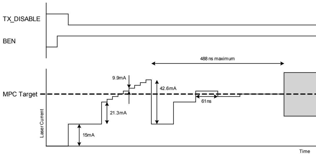
Figure 39 - Closed Loop Fast Start-up Algorithm Example
