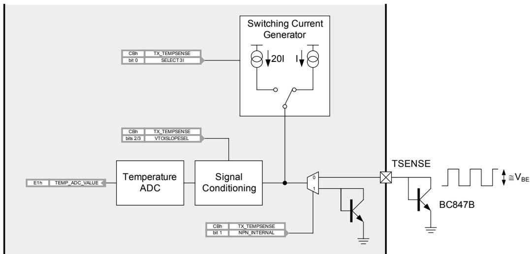
Figure 17 – Temperature sensor functional block diagram
