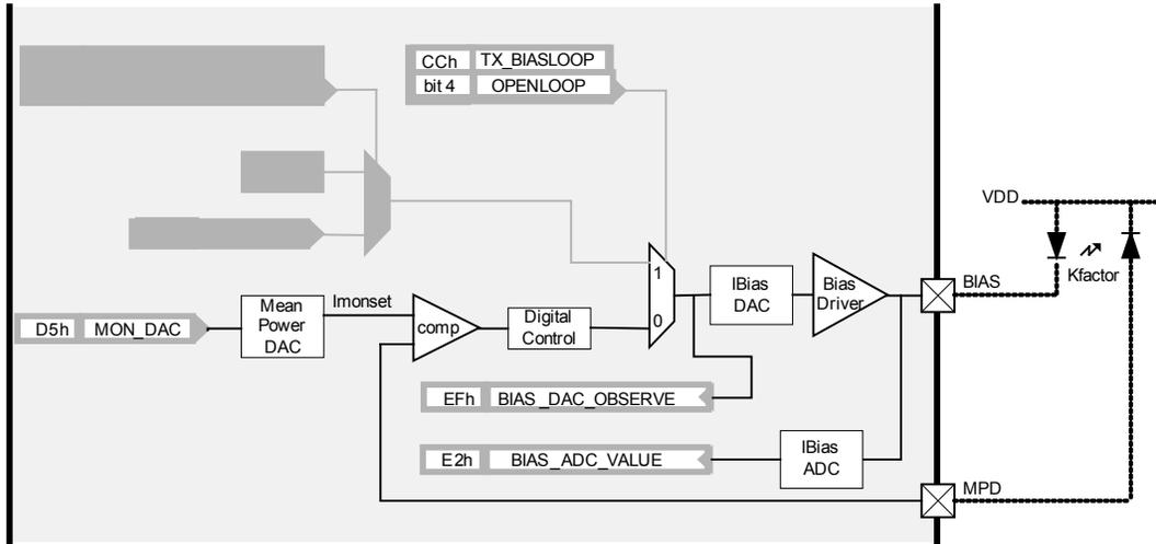
Figure 14 - Bias Current Generation, Closed Loop
