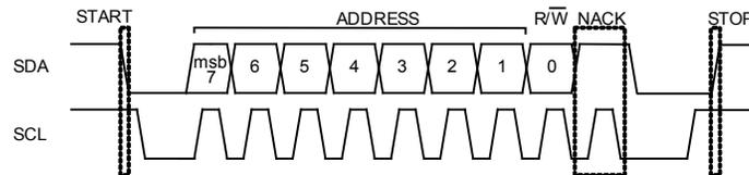
Figure 22 - Address decoding example – slave not available
