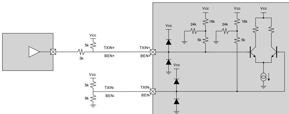
Figure 36 – Single-ended CMOS/LVTTL interface for BEN
