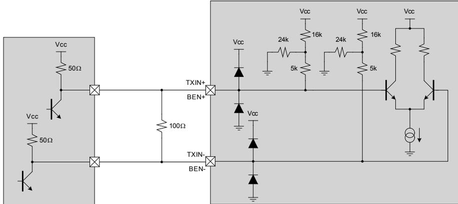
Figure 34 - DC-Coupled CML interface for TXIN and BEN
