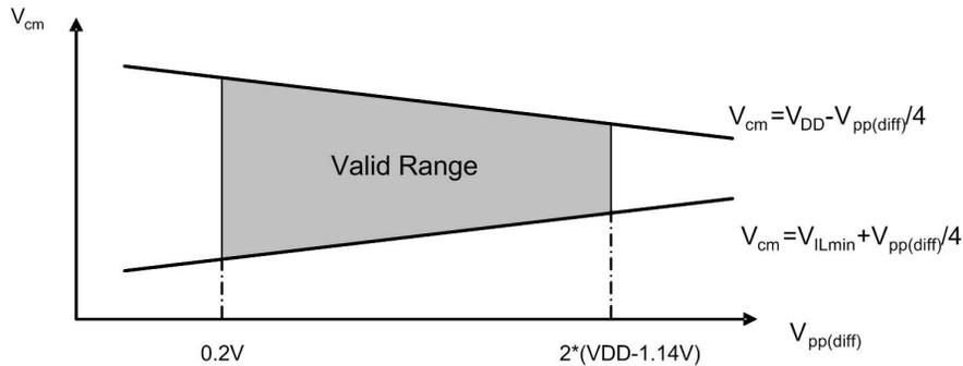
Figure 4 – Valid combinations of transmitter input voltages
