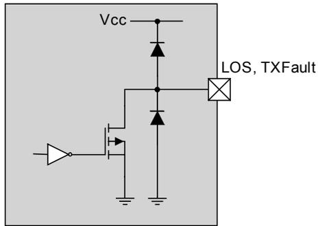
Figure 31 - LOS/TX\_FAULT output
