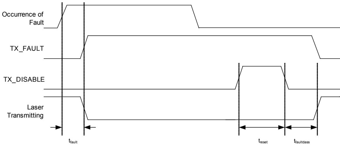
Figure 6 - Fault detection
