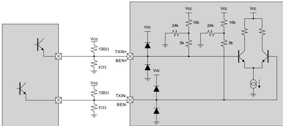
Figure 35 - DC-Coupled LVPECL interface for TXIN and BEN
