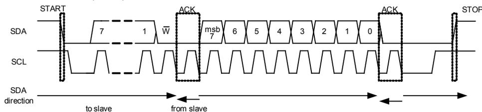
Figure 23 - Write transaction
