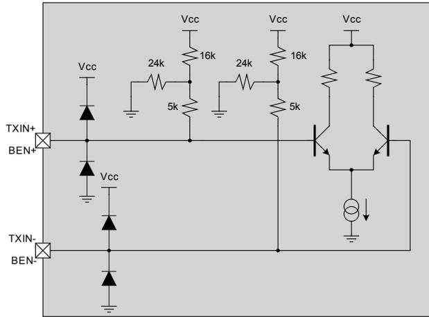
Figure 25 - Transmit input structure
