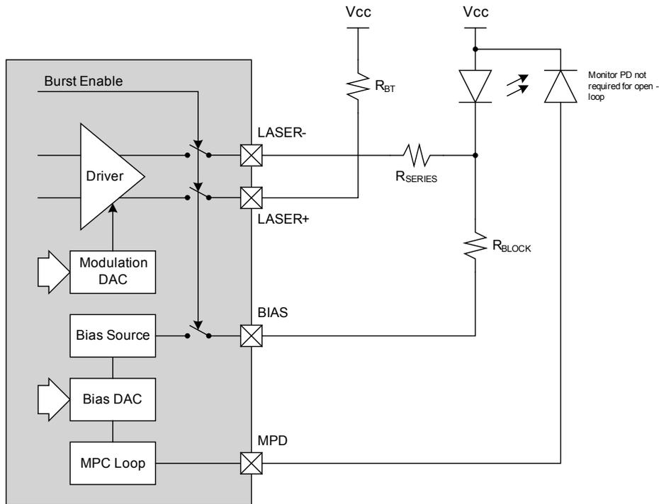
Figure 37 - DC-Coupled Laser Application Diagram
