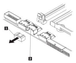
b. Connect the RAID level-5 enabler plug (that came with the system) 1 to the SAS/SATA backplane 1 connector on the system board.
