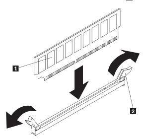
11. Firmly press the DIMM straight down into the connector by applying pressure on both ends of the DIMM simultaneously. The retaining clips snap into the locked position when the DIMM is firmly seated in the connector. If there is a gap between the DIMM and the retaining clips, the DIMM has not been correctly installed. Open the retaining clips, remove the DIMM, and then reinsert it.
