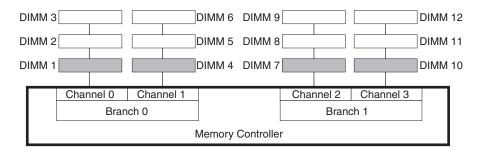
The server can operate in two major modes: mirroring and non-mirroring (normal). The server can also operate in a single-channel mode when one DIMM is installed.
