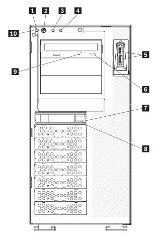
System power LED CD-eject or DVD-eject button 7 2 Power-control button Hot-swap hard disk drive status LED (amber) 3 Hard disk drive activity LED 8 Hot-swap hard disk drive activity LED (green) System-error LED CD or DVD drive activity LED (green) 9 5 **USB** connectors 10 Front information panel
