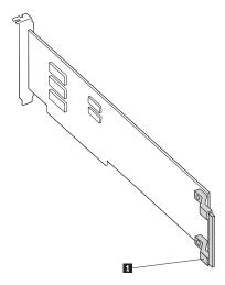
9. Carefully grasp the adapter 2 by the top edge or upper corners, and align it with the expansion slot guides; then, press the adapter firmly into the expansion slot. Move the adapter directly from the static-protective package to the expansion slot.
