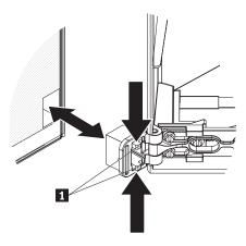
**Note:** The bezel also will disengage from the chassis hinges if you rotate the bezel beyond 180° or if excessive pressure is applied to the bezel. Do not be alarmed because this is how the bezel was designed. The bezel is designed with breakaway hinges so that you can easily reattach it to the chassis. Press the retention tabs 1 on the hinge assembly toward each other and pull the hinge assembly out of the chassis.
