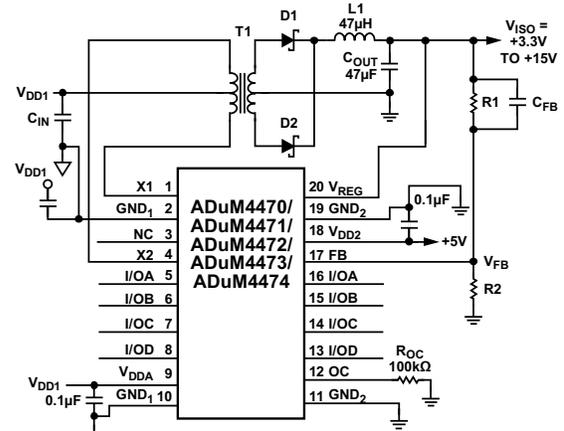
$V_{ISO} = V_{FB} \times (R1 + R2)/R2$
