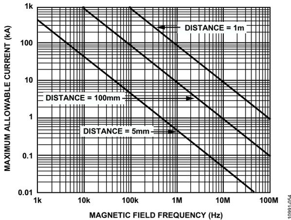
Figure 54. Maximum Allowable Current for Various Current-to-ADuM447x Spacings
