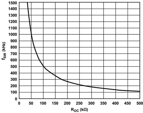
Figure 13. Switching Frequency ( $f_{sw}$ ) vs.  $R_{OC}$  Resistance
