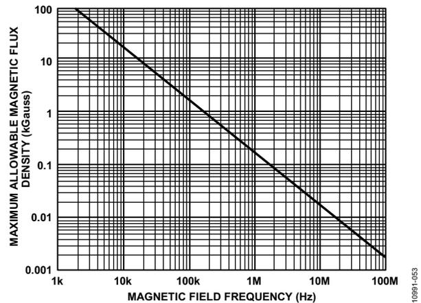
Figure 53. Maximum Allowable External Magnetic Flux Density
