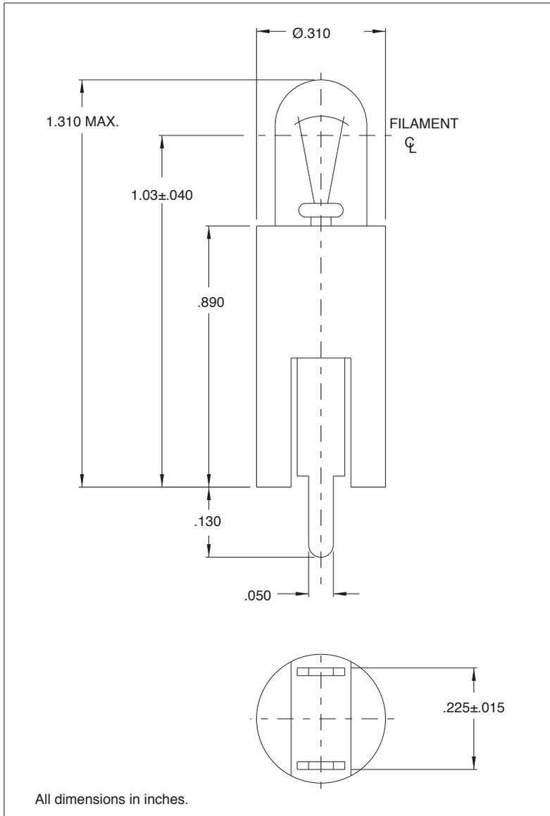
Mounting: Printed circuit Board
