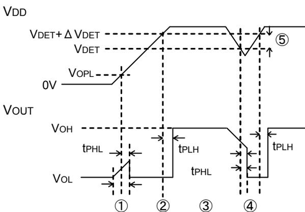
Fig.14 Timing Waveform
