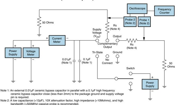
Note 4: A 10 ohm to 33 ohm series resistor is required to limit overshoot. Rs value is circuit layout dependant.
