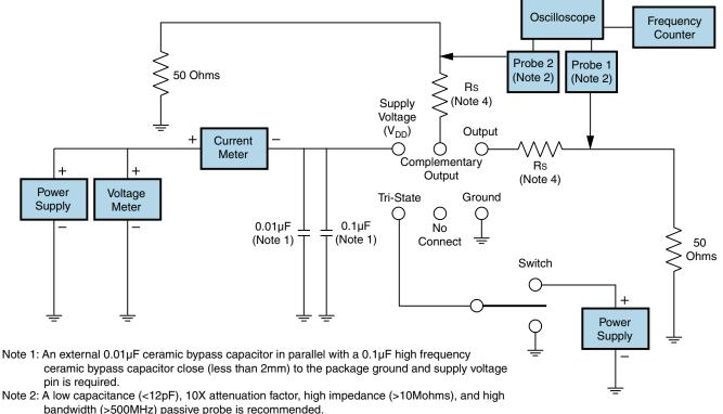
Note 3: Test circuit PCB traces need to be designed for a characteristic line impedance of 50 ohms.
