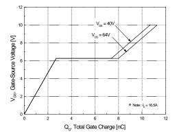
Figure 6. Gate Charge Characteristics
