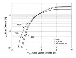
Figure 2. Transfer Characteristics
