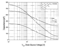
Figure 5. Capacitance Characteristics
