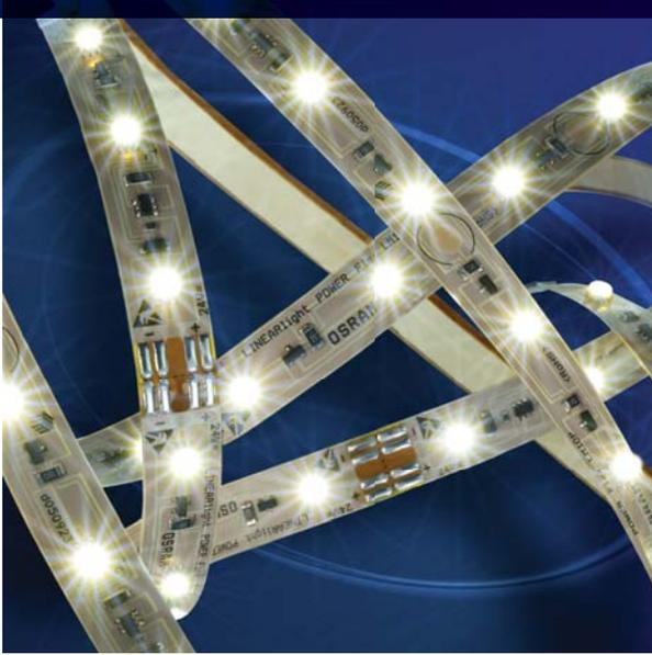
LINEARlight POWER FLEX LED modules are suitable alternatives to conventional sources used in linear and curved architecture and display lighting applications. The module consists of high brightness, white LEDs uniformly spaced on a flexible, self adhesive substrate.
