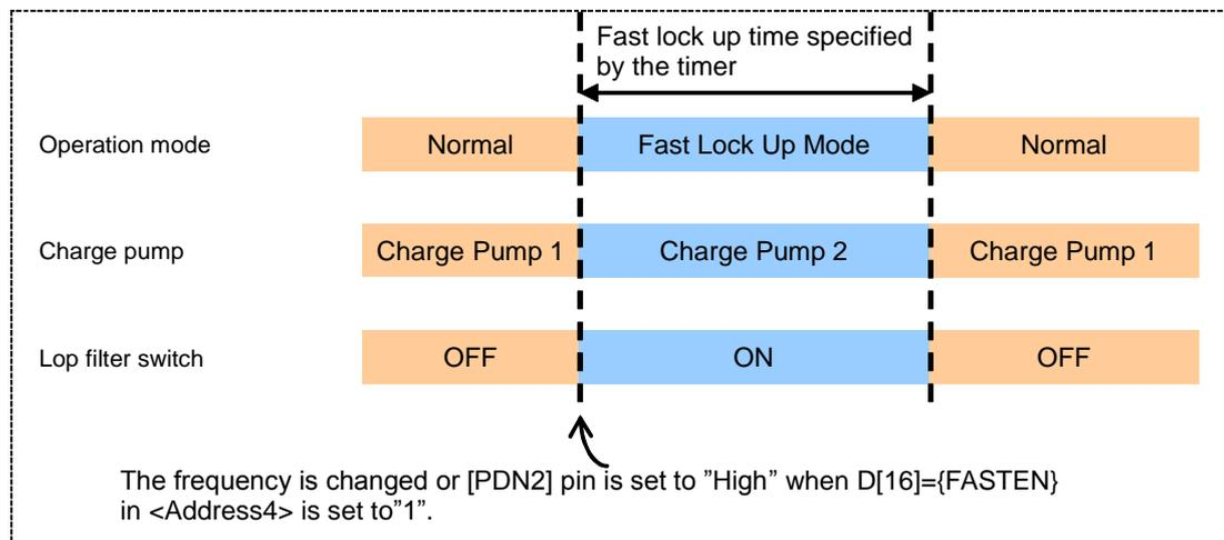
**Fig. 6 Timing Chart for Fast Lock Up Mode**
