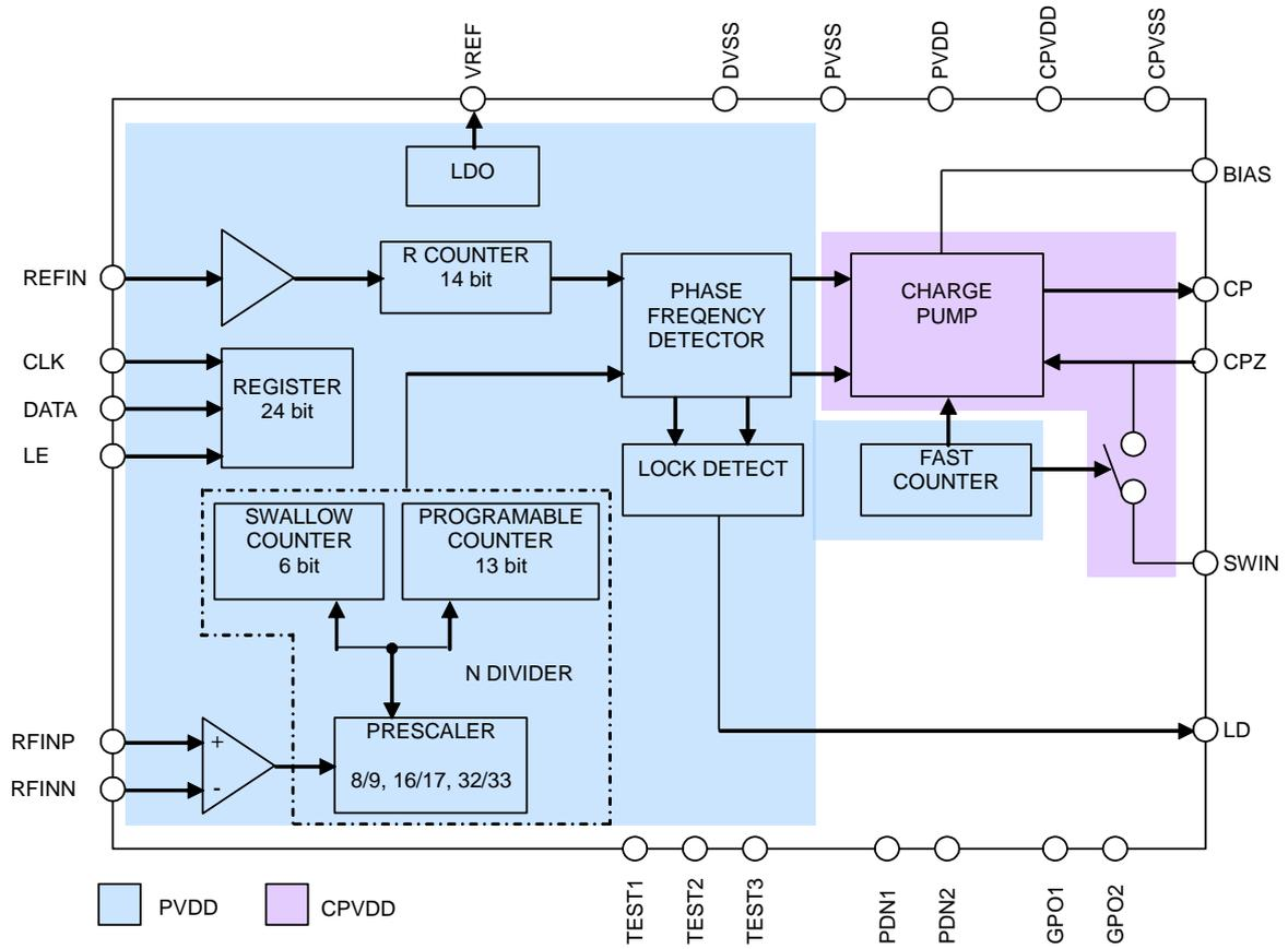
**Fig. 15 Power Supply Block Diagram**
