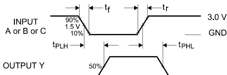
**Figure 1. Switching Waveforms**
