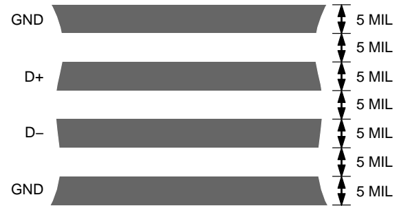
Figure 12. Typical Assignment of Signal Tracks
