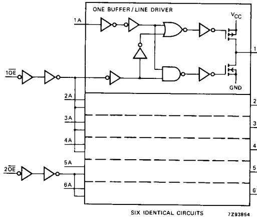
Fig. 5 Logic diagram.
