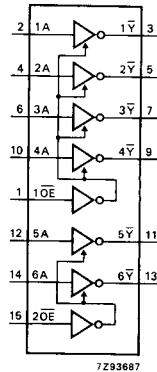
Fig. 4 Functional diagram.
