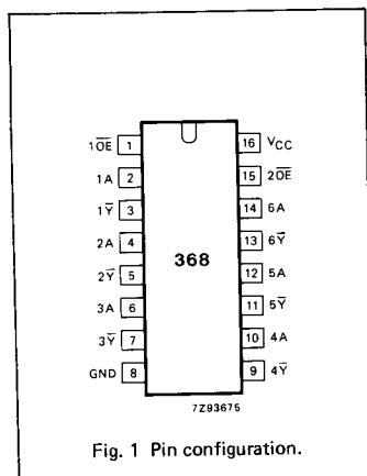
Fig. 1 Pin configuration.
