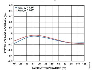
Figure 13. System Voltage Accuracy vs. Ambient Temperature,  $Load = 100 \text{ mA}, V_{VINx} = 5.5 \text{ V}$
