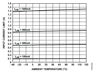
Figure 19. Input Current Limit vs. Ambient Temperature
