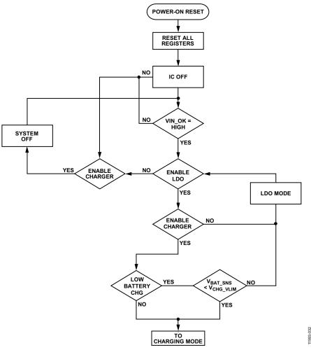
Figure 29. Simplified Battery and VINx Connect Flowchart
