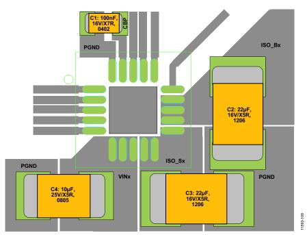
Figure 38. Reference PCB Floor Plan
