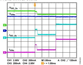
Figure 20. Charging Startup,  $V_{VINx} = 5.0 V$ , ILIM[3:0] = 0110 (Binary) = 500 mA, ICHG[4:0] = 01110 (Binary) = 750 mA
