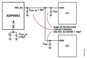
Figure 36. Splitting ISO\_Sx Capacitance
