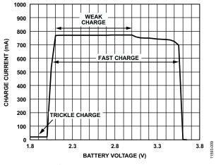
Figure 6. Battery Charge Current vs. Battery Voltage, ICHG[4:0] = 01001 (Binary) = 500 mA, ILIM[3:0] = 1111 (Binary) = 2100 mA
