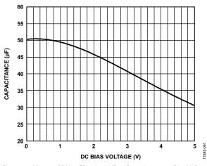
Figure 35. Murata GRM31CR61A226KE19 Capacitance vs. Bias Voltage
