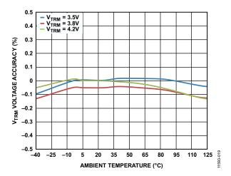
Figure 16. Termination (V<sub>TRM</sub>) Voltage Accuracy vs. Ambient Temperature
