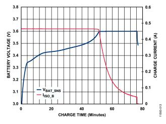
Figure 10. Charge Profile, ILIM[3:0] = 0110 (Binary) = 500 mA, LiFePO₄ Battery Capacity = 500 mAh
