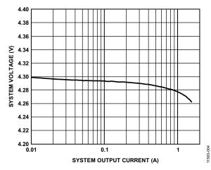
Figure 4. System Voltage vs. System Output Current, LDO Mode, VSYSTEM[2:0] = 000 (Binary) = 4.3 V
