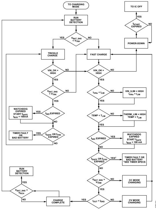
Figure 30. Simplified Charging Mode Flowchart
