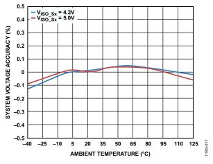
Figure 14. System Voltage Accuracy vs. Ambient Temperature, Trickle Charge Mode,  $V_{ISO\_Sx} = 4.3 \ V$  and  $V_{VINx} = 5.0 \ V$ , or  $V_{ISO\_Sx} = 5.0 \ V$  and  $V_{VINx} = 6.0 \ V$
