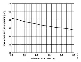
Figure 7. Ideal Diode  $R_{ON}$  vs. Battery Voltage,  $I_{ISO\_Sx} = 500$  mA, VINx Open
