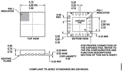
Figure 39. 20-Lead Lead Frame Chip Scale Package [LFCSP\_WQ] 4 mm × 4 mm Body, Very Very Thin Quad (CP-20-8) Dimensions shown in millimeters
