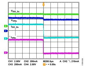
Figure 23. USB VBUS Disconnection
