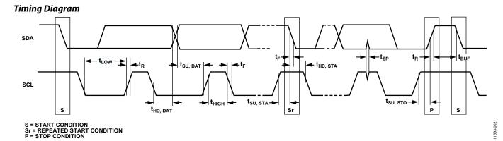
Figure 2. I<sup>2</sup>C Timing Diagram
