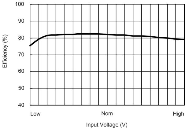
**Efficiency vs Input Voltage ( Single Output )**
