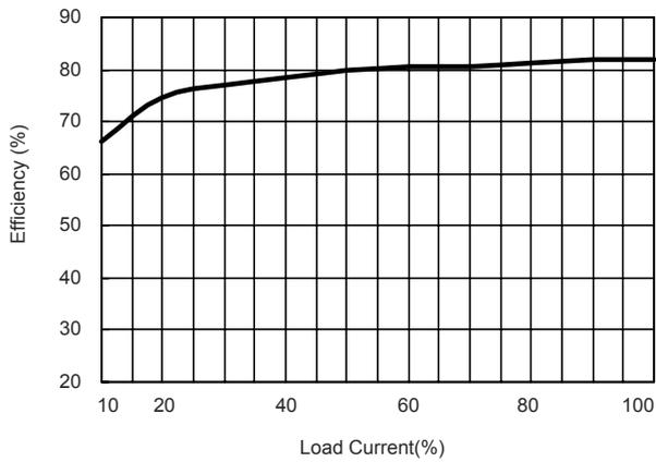
**Efficiency vs Output Load ( Single Output )**
