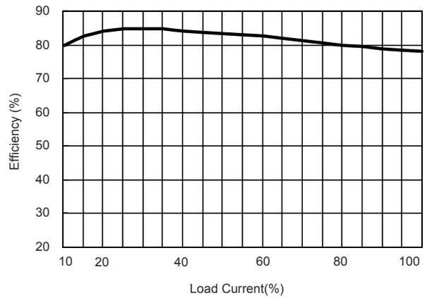
**Efficiency vs Output Load ( Dual Output )**
