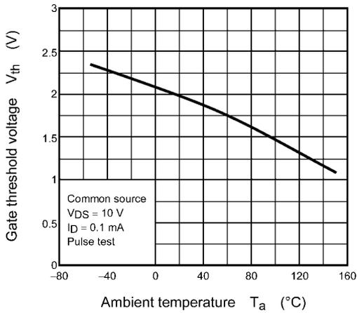
**Fig. 8.2.9  $V_{th} - T_a$**
