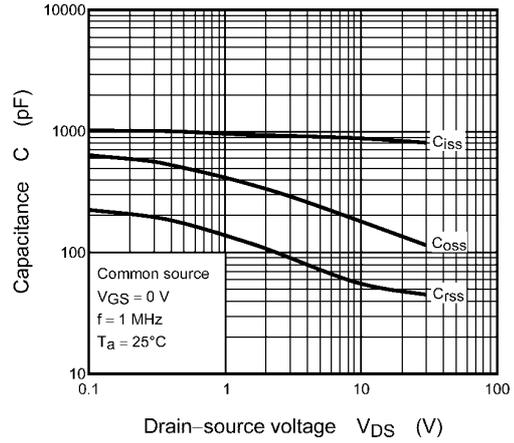
**Fig. 8.2.8 Capacitance -  $V_{DS}$**
