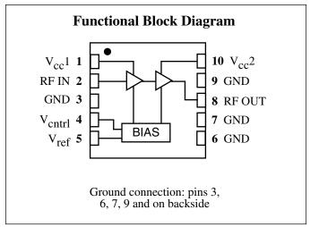
fixed positive voltage and requires no external matching which significantly reduces space, cost and enhances ease of use. A current adjustment pin (Vcntrl) is provided to improve efficiency for the low RF power range of operation.
