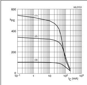
**TR1 (NPN)**;  $V_{CE} = 5 \text{ V}$ .
