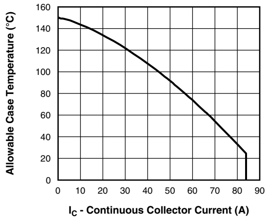
Fig. 1 - Maximum DC IGBT Collector Current vs. Case Temperature
