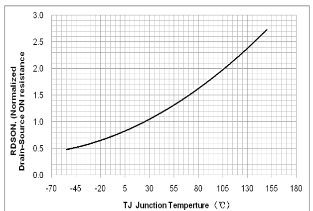
Fig. 6. On resistance variation vs. junction temperature
