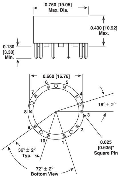
\*Shows typical pin spacing. Pin #10 is omitted on all models except -05, -06, -12.
