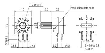
Unless otherwise specified, tolerance:  $\pm$  0.3 (Unit: mm)
