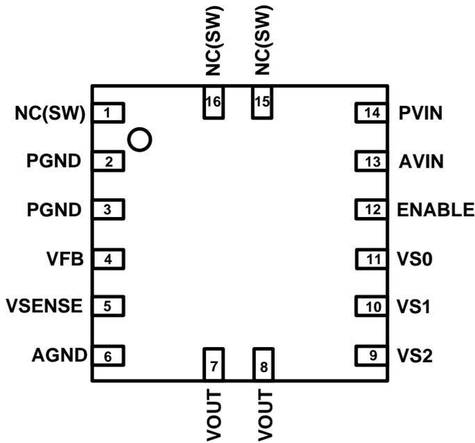
Figure 3. EP53A8LQA Pin Out Diagram (Top View)
