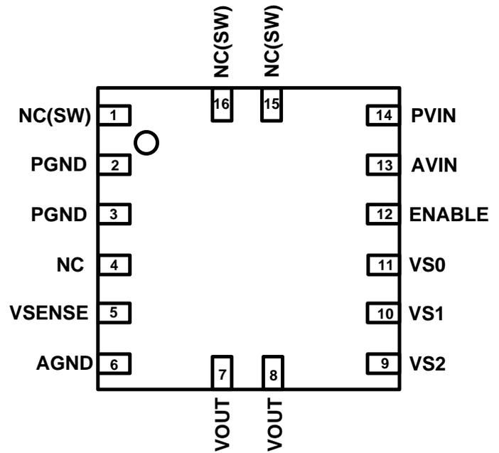
Figure 4. EP53A8HQA Pin Out Diagram (Top View)
