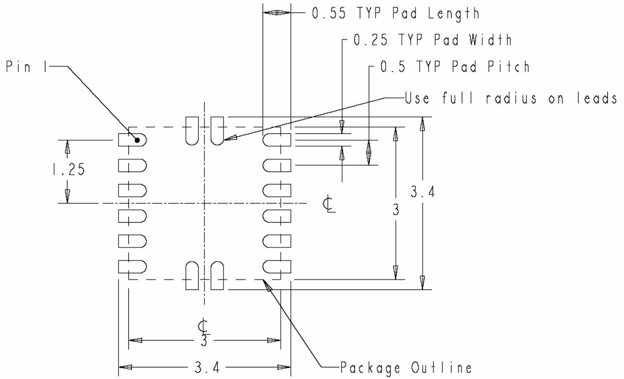
Figure 11. EP53A8xQA PCB Footprint (Top View)
