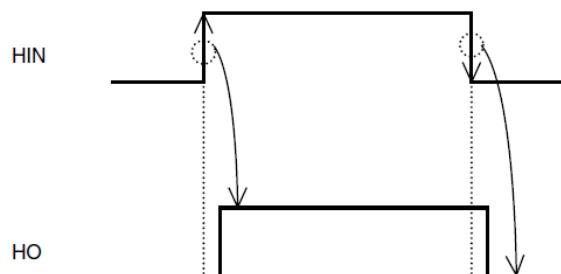
**HIGH VOLTAGE HALF BRIDGE DRIVER****TIMING DIAGRAM****1. Input/Output Timing Diagram**
