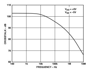
Figure 8. Crosstalk vs. Frequency
