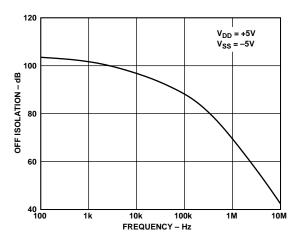
Figure 6. Off Isolation vs. Frequency
