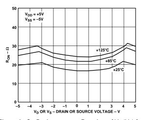
Figure 2. On Resistance as a Function of  $V_D \left( V_S \right)$  for Different Temperatures
