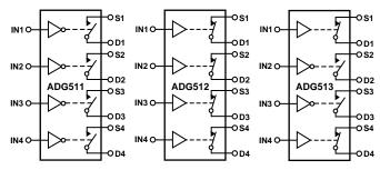
SWITCHES SHOWN FOR A LOGIC "1" INPUT
