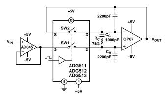
Figure 9. Accurate Sample-and-Hold
