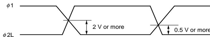
**Remark** Adjust cross points (φ 1, φ 2), (φ 1L, φ 2) and (φ 1, φ 2L) with input resistance of each pin.
