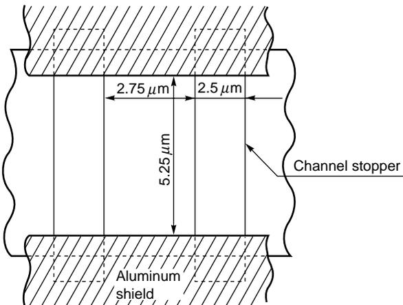
**PHOTOCELL ARRAY STRUCTURE DIAGRAM (Line spacing)**
