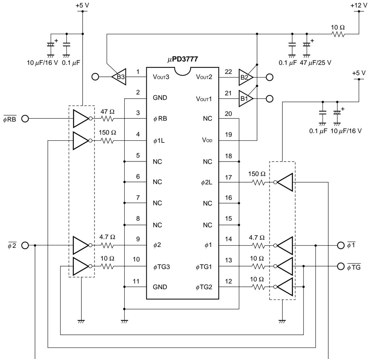
**Remark** The inverters shown in the above application circuit example are the 74HC04 (data rate < 2 MHz) or the 74AC04 (data rate: 2 to 4 MHz).
