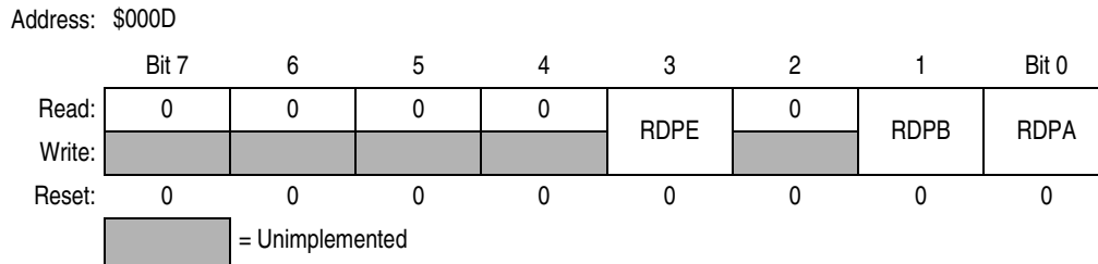
Figure 6-9. Reduced Drive of I/O Lines (RDRIV)
