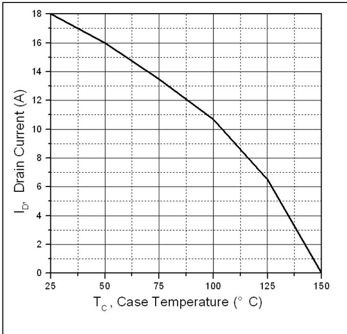
Figure 5. Maximum Drain Current Vs. Case Temperature
