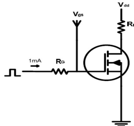
**Switch Time Test Circuit:**
