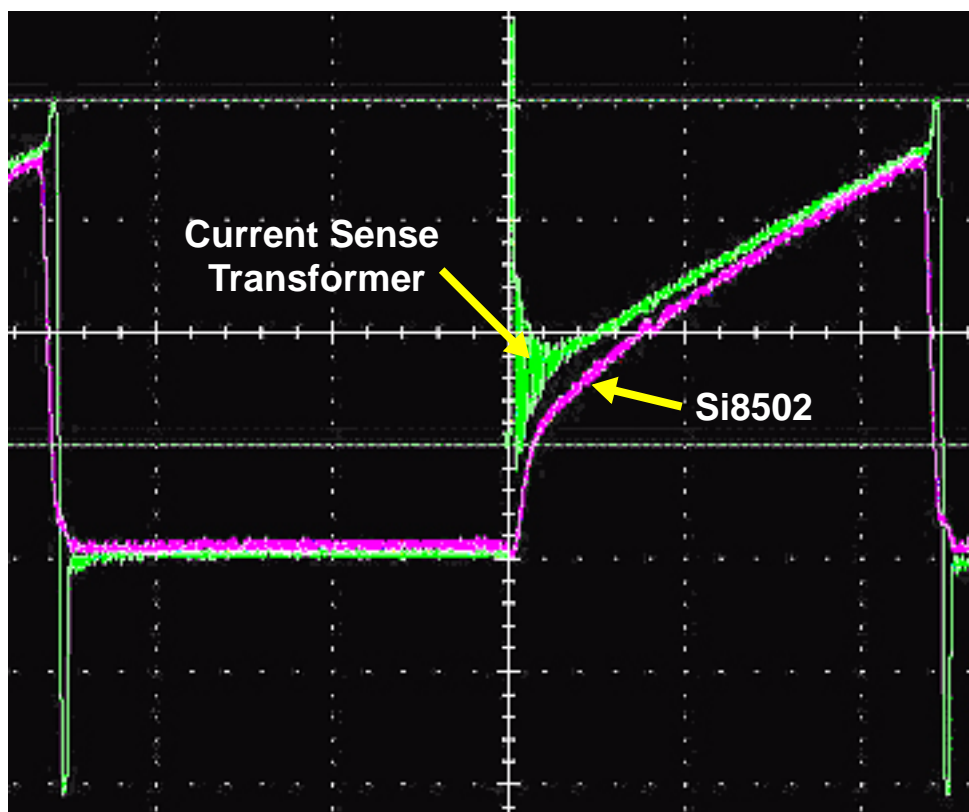
Figure 8. Leading-Edge Noise Suppression Waveforms (200 kHz, 9.3A Load) (Si8502 waveform measured directly on OUT pin with no external filter)
