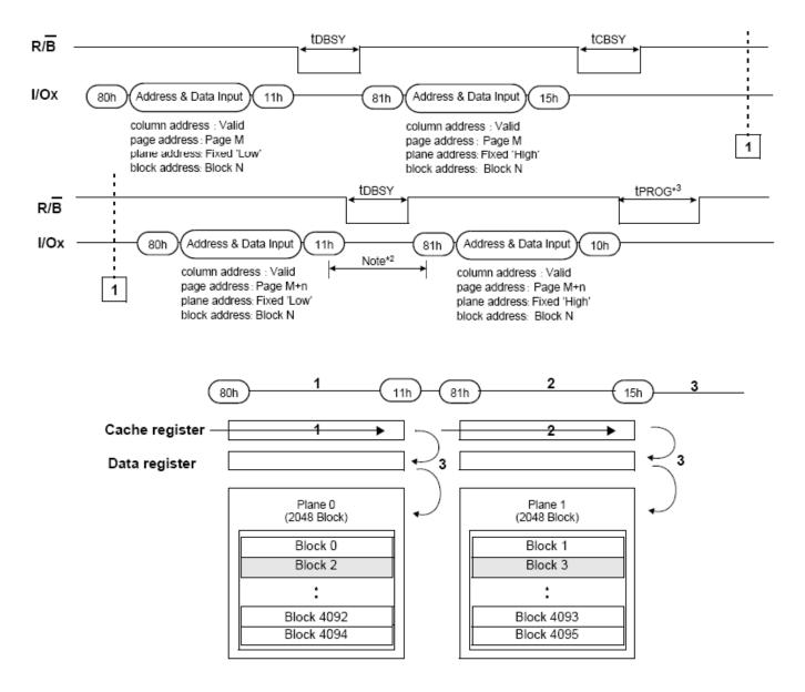
NOTE : 1. It is noticeable that same row address except for A20 is applied to the two blocks
