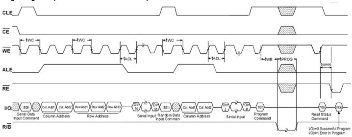
**NOTE:**  $t_{ADL}$  is the time from the  $\overline{WE}$  rising edge of final address cycle to the  $\overline{WE}$  rising edge of the first data cycle.
