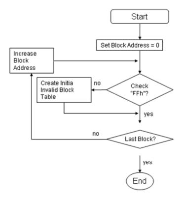
Check "FFh" at the 1st Byte column address in the spare area of the 1st and 2nd page in the block.
