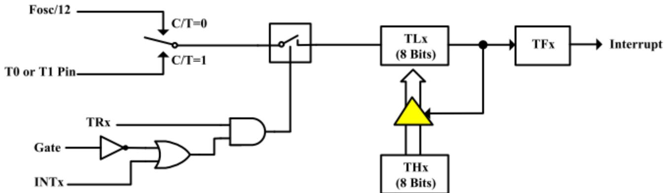
Fig. 6-3: Mode 2 8-bit auto-reload Counter/Timer operation.
