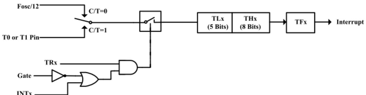
Fig. 6-1: Mode 0 -13 bit Timer / counter operation
