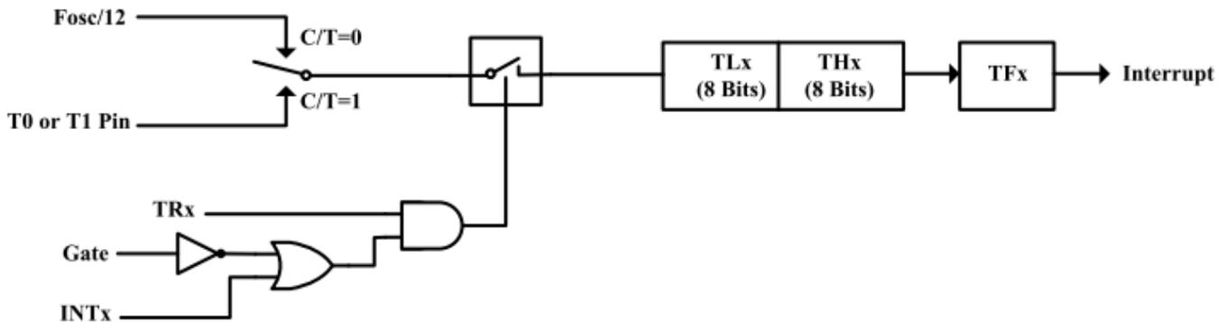
Fig. 6-2: Mode 1 16 bit Counter/Timer operation
