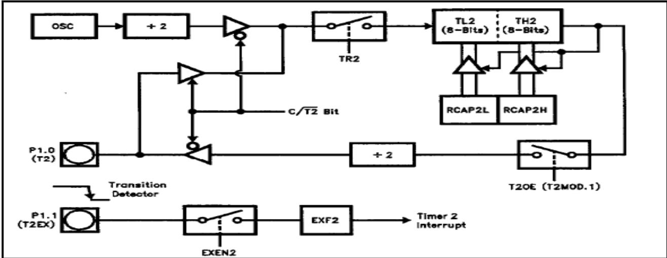
Fig. 7-4 : Timer 2 in clock-out mode
