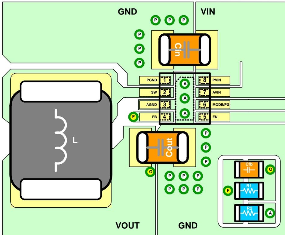
Figure 20. Recommended PCB Layout for Application Boards
