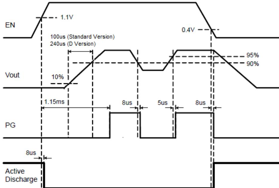
Figure 19. Power Good and Active Discharge Timing Diagram
