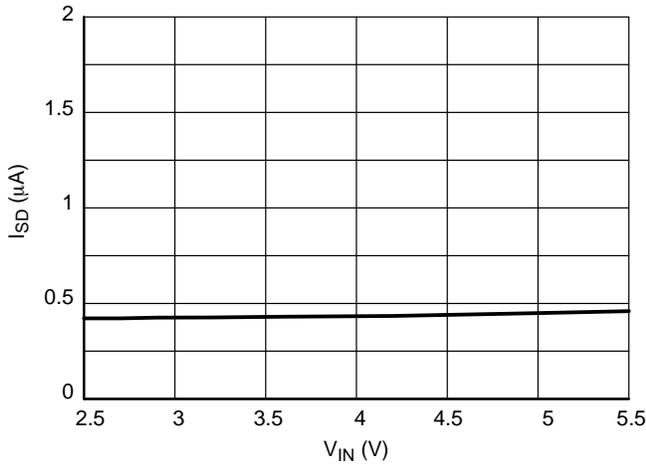
Figure 3. Shutdown Current vs. Input Voltage (EN = Low, T<sub>A</sub> = 25°C)
