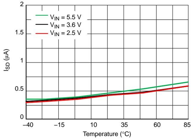
Figure 4. Shutdown Current vs. Temperature (EN = Low, V<sub>IN</sub> = 3.6 V)
