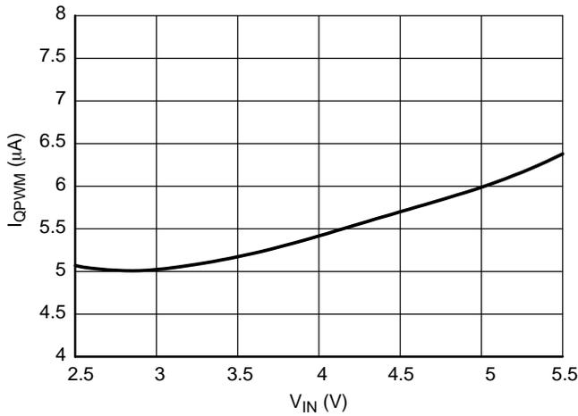
Figure 5. PWM Quiescent Current vs. Input Voltage (EN = High, Open Loop, V<sub>OUT</sub> = 1.8 V, T<sub>A</sub> = 25°C)
