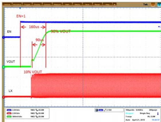
Figure 17. Soft-start Time for NCV6323 ( $V_{IN} = 4.2\text{ V}$ ,  $V_{OUT} = 1.8\text{ V}$ ,  $I_{OUT} = 0\text{ A}$ ,  $L = 1\ \mu\text{H}$ ,  $C_{OUT} = 10\ \mu\text{F}$ )
