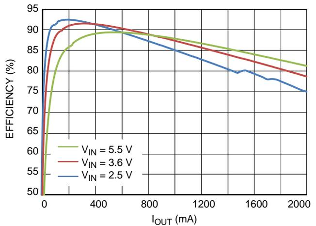
Figure 8. Efficiency vs. Output Current and Input Voltage (V<sub>OUT</sub> = 1.8 V, T<sub>A</sub> = 25°C)
