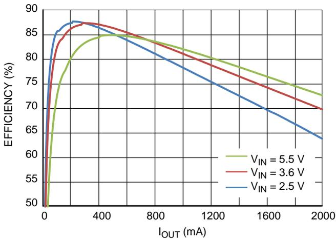
Figure 7. Efficiency vs. Output Current and Input Voltage (V<sub>OUT</sub> = 1.05 V, T<sub>A</sub> = 25°C)
