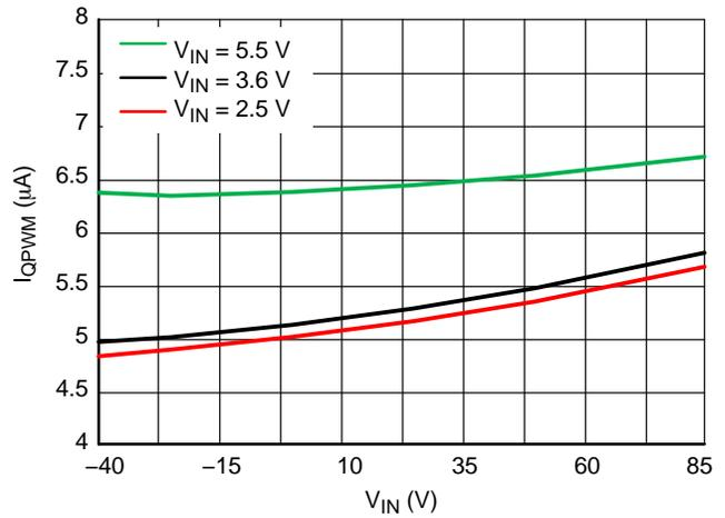
Figure 6. PWM Quiescent Current vs. Temperature (EN = High, Open Loop, V<sub>OUT</sub> = 1.8 V, V<sub>IN</sub> = 3.6 V)
