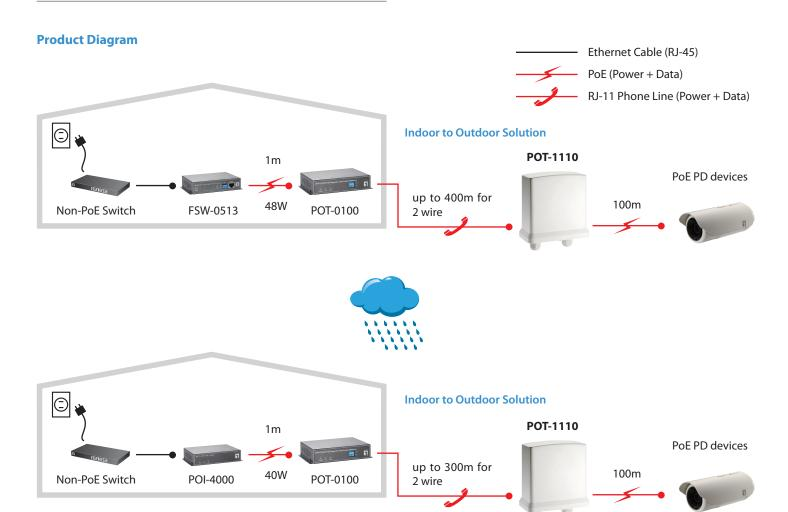
Note: These distances are typical results when used with 24AWG RJ-11 Cable
