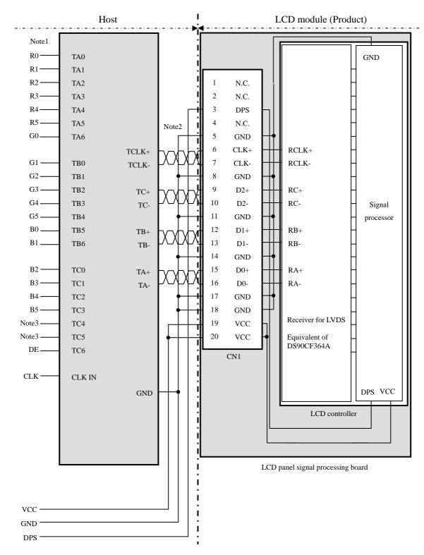
Note1: LSB (Least Significant Bit) – R0, G0, B0 MSB (Most Significant Bit) – R5, G5, B5
