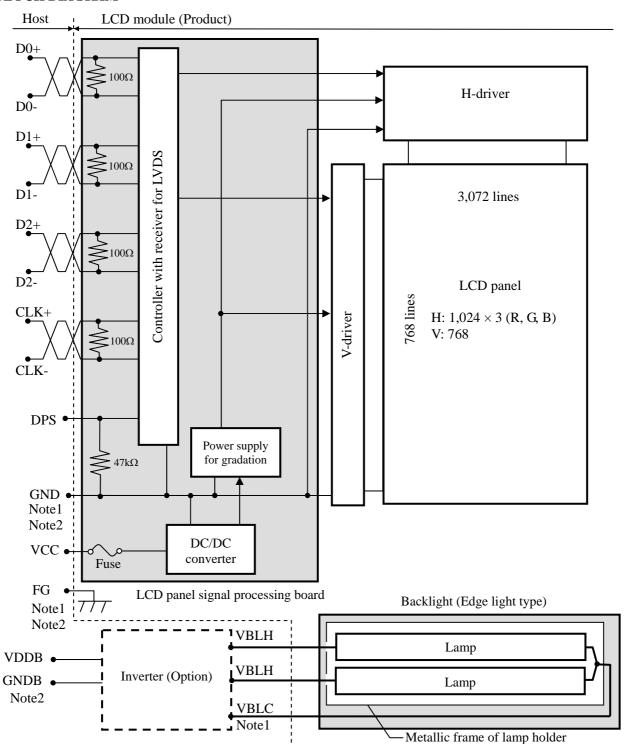
Note1: Relations between GND (Signal ground), FG (Frame ground) and VBLC (Lamp low voltage terminal) in the LCD module are as follows.
