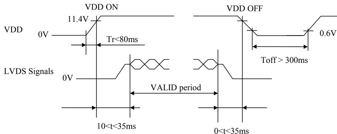
Note1: LVDS signals should be measured at the terminal of 100Ω resistor.
