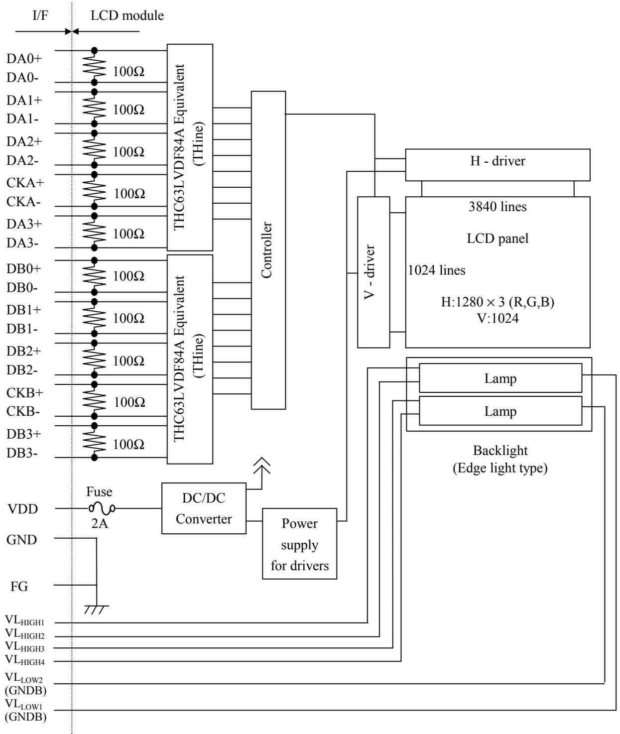
Note1: GND (Signal Ground) is connected to FG (Frame Ground) in the LCD module. Neither GND nor FG is connected to GNDB (Backlight Ground). These grounds should be connected to system ground in customer equipment.
