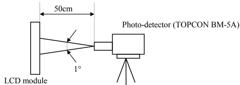
Note 2: Viewing angle is  $\theta_x = \pm 0^\circ, \theta_y = \pm 0^\circ$ , at center
