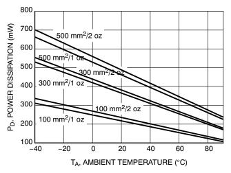
Figure 6. Power Dissipation vs. Ambient Temperature @  $T_J = 150$ °C
