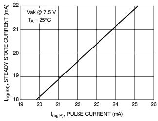
Figure 4. Steady State Current vs. Pulse Current Testing
