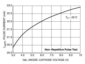
Figure 3. Pulse Current  $(I_{reg(P)})$  vs. Anode-Cathode Voltage (Vak)
