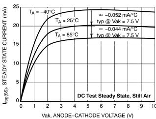
Figure 2. Steady State Current  $(I_{reg(SS)})$  vs. Anode–Cathode Voltage (Vak)
