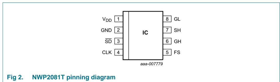
Fig 2. NWP2081T pinning diagram
