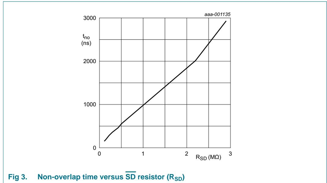
**Fig 3. Non-overlap time versus  $\overline{SD}$  resistor ( $R_{SD}$ )**
