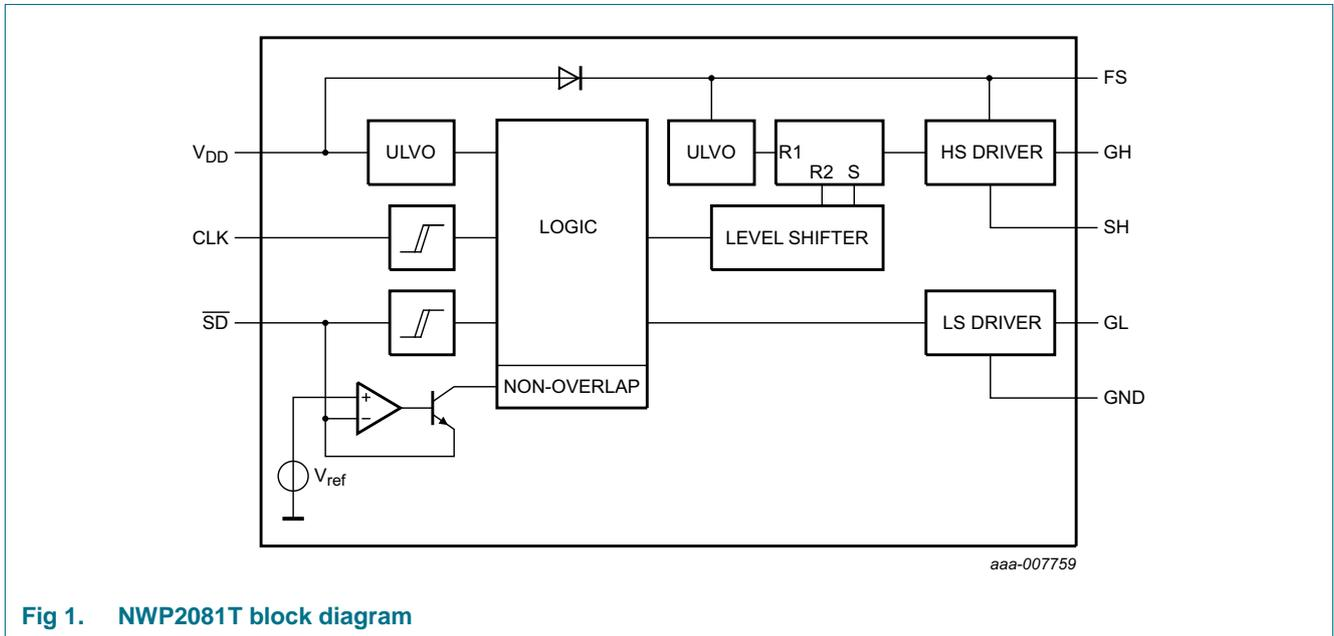
Fig 1. NWP2081T block diagram
